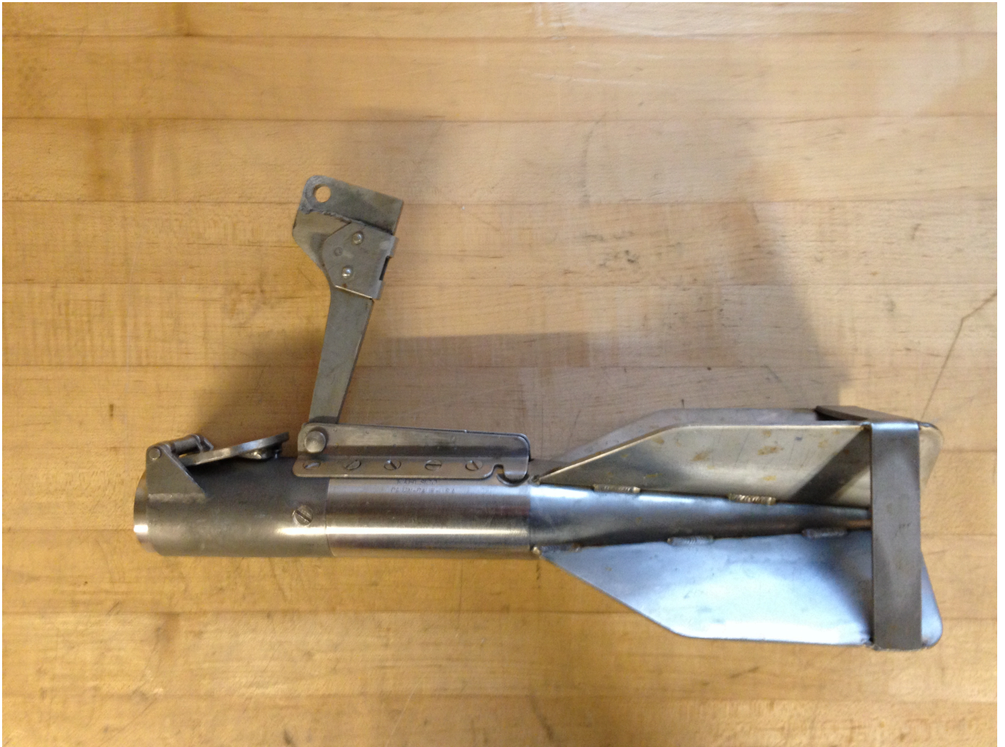
Figure 12: Torpedo style grab sampler used about NOAA Ship Fairweather launches.
