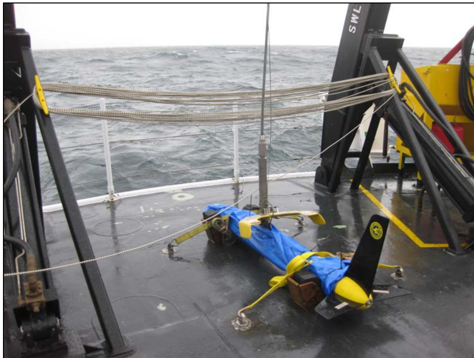
Figure 7: Towed Klein 5000 Side Scan Sonar on Fairweather
