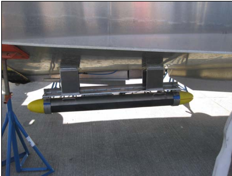
Figure 7: Hull-Mounted Klein 5000 Side Scan Sonar on Fairweather Launch with TPU
