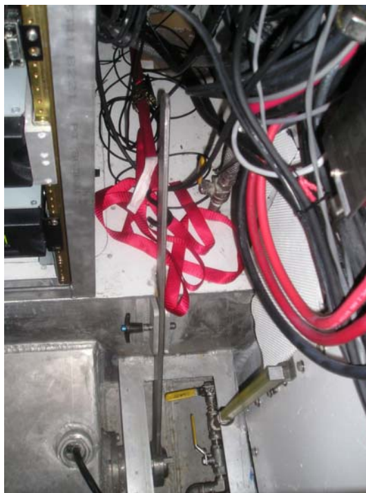
Figure 9: The deployment lever arm, set pin and ratcheting tie-down strap. The pin was eventually removed to allow the arm to reach the under hull stop.
