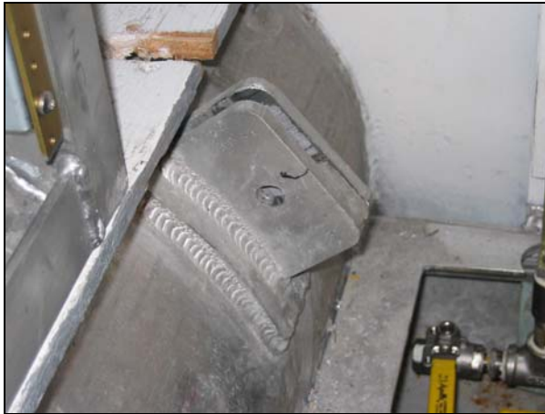
Figure 7: Aluminum bracket for locking position transducer down
