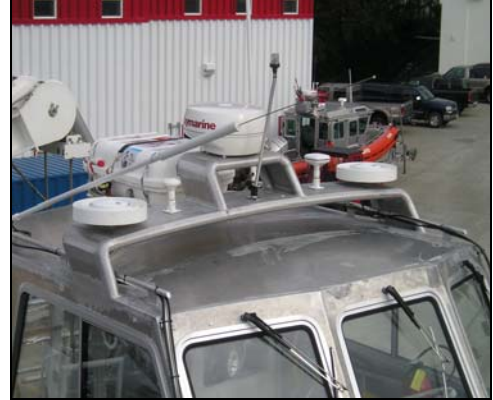
Figure 8: POS/MV antennas mounted on 1010 (side view)
