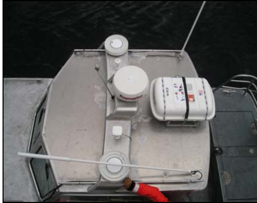
Figure 7: POS/MV antennas mounted on 1018 (top view)
