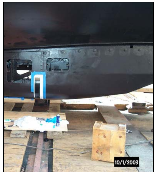
Figure 2: RESON SeaBat 8111ER MBES on FAIRWEATHER
