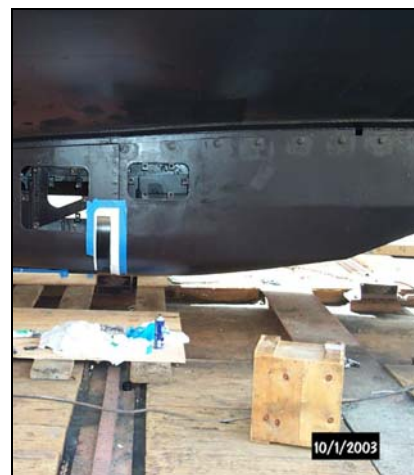
Figure 2: RESON SeaBat 8111ER MBES on FAIRWEATHER
