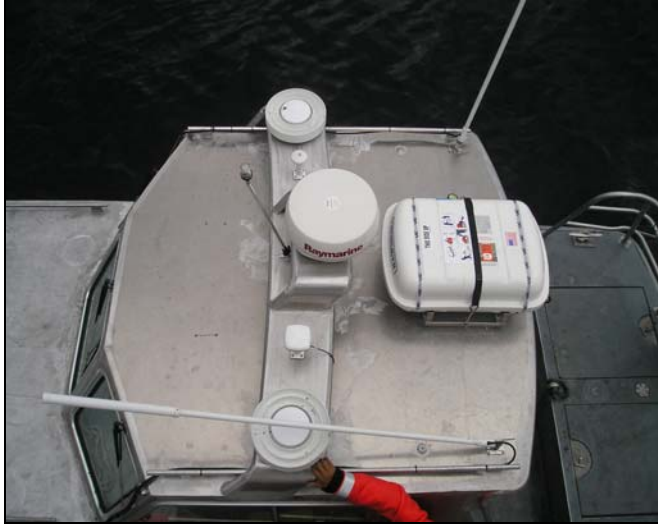
Figure 5: POS/MV antennas mounted on 1018 (top view)
