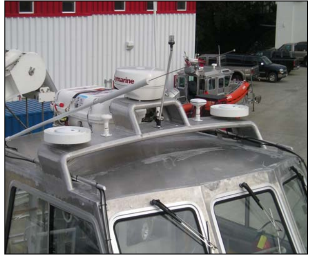
Figure 6: POS/MV antennas mounted on 1010 (side view)
