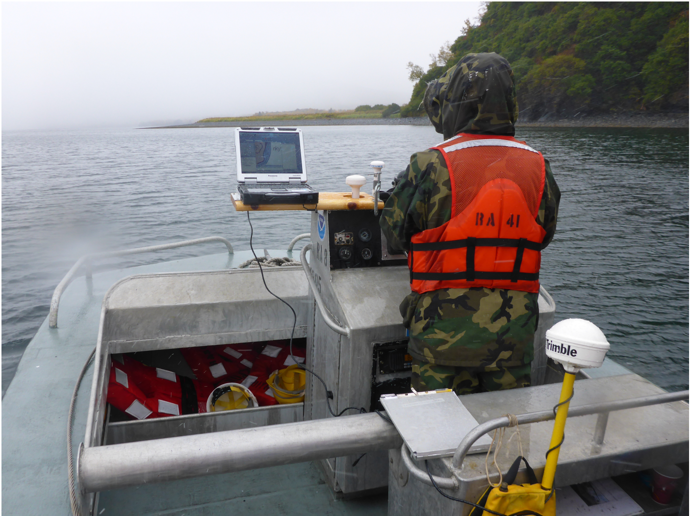
Figure 30: Survey skiff RA8 collecting the along-shore buffer line using a Trimble GPS backpack system connected to a Toughbook computer.
