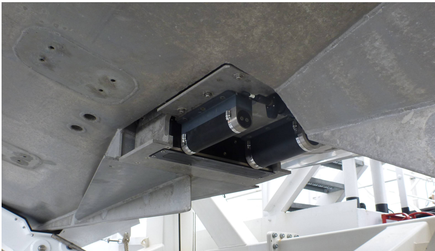
Figure 10: Reson SeaBat 7125-B mounted on survey launch 2801.
