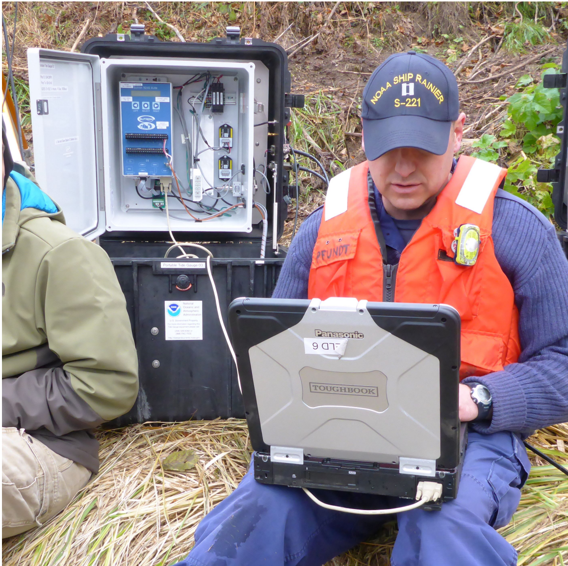
Figure 19: Downloading data from the Portable Tide Gauge (PTG) system, 9210B data collection platform.
