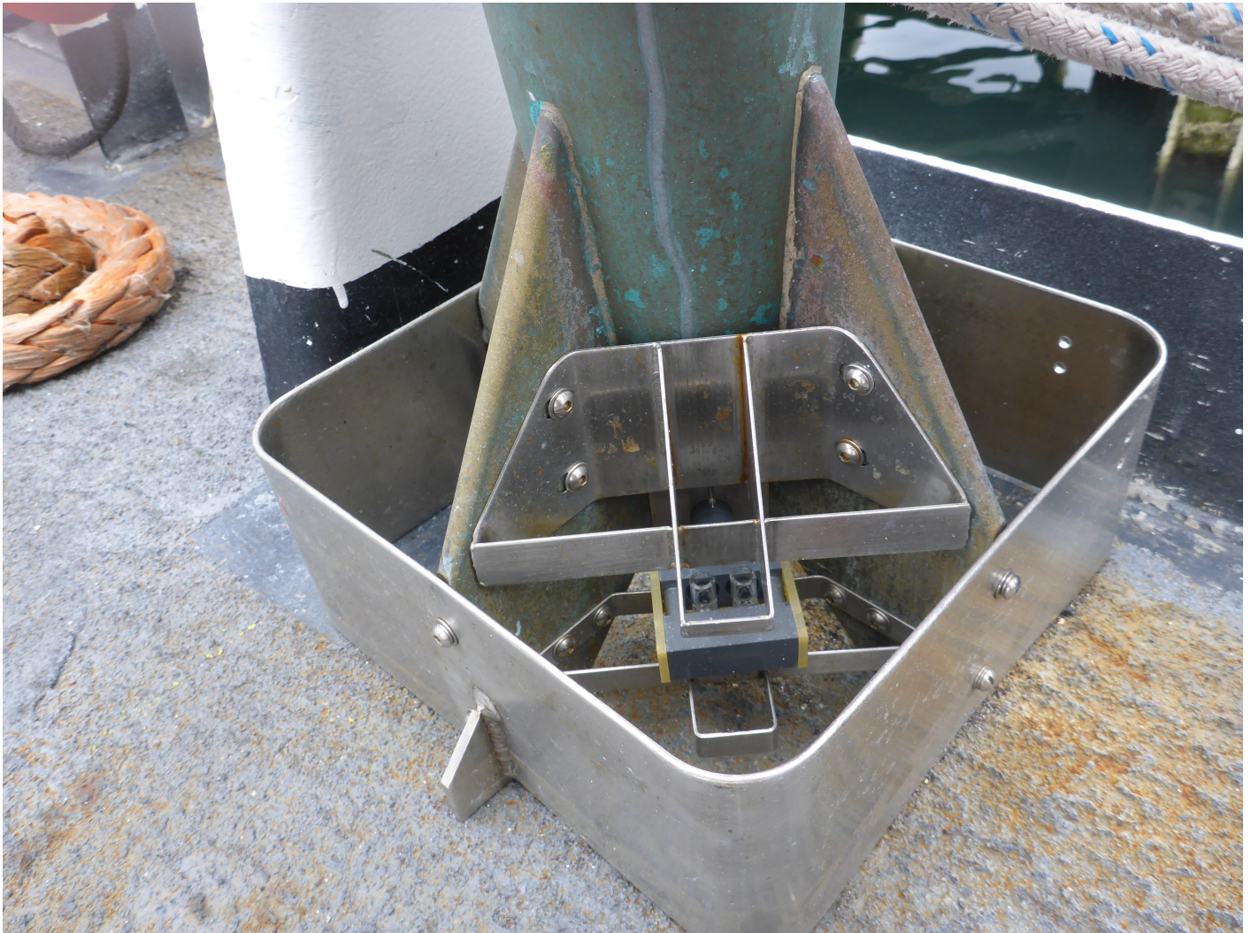
Figure 16: The stainless steel sensor guards as installed on the MVP200 fish.
