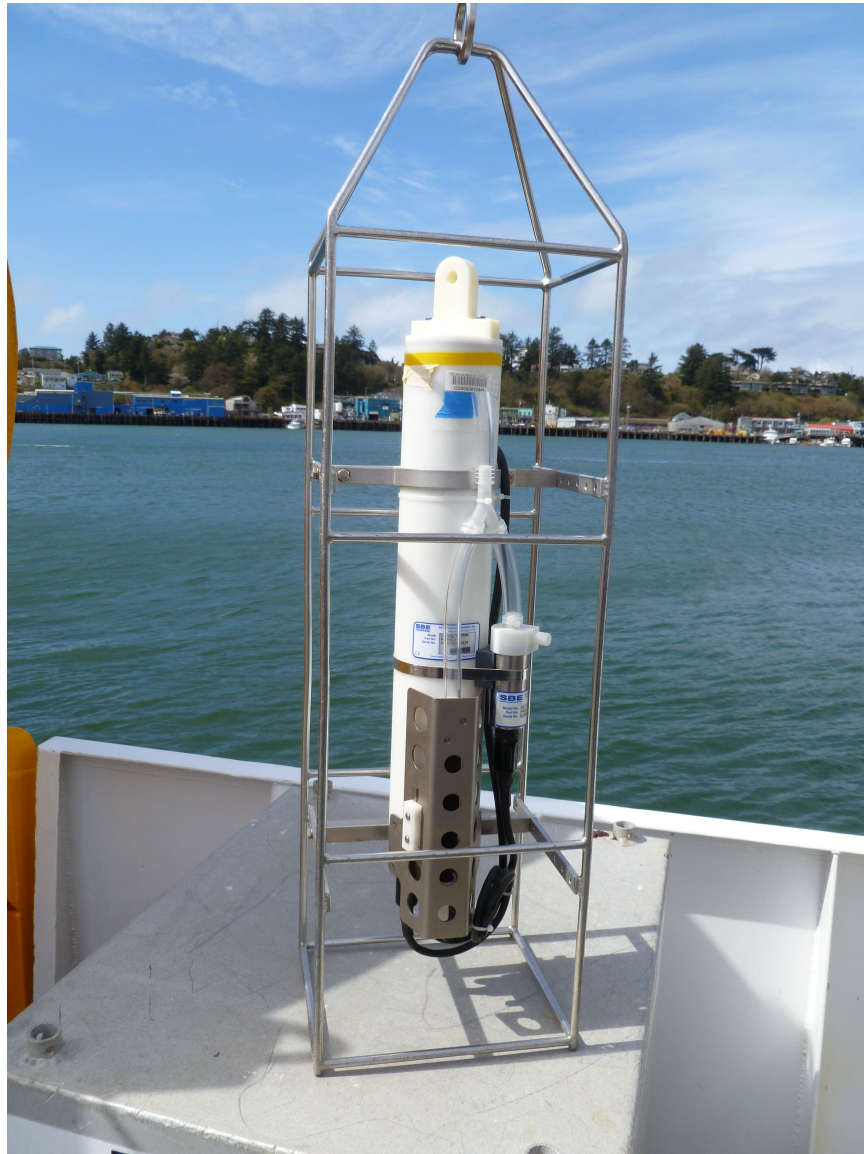
Figure 14: The SBE 19plus SEACAT profiler. Note the band of electrical tape around the housing at the top of profiler marking this as the "yellow" CTD
