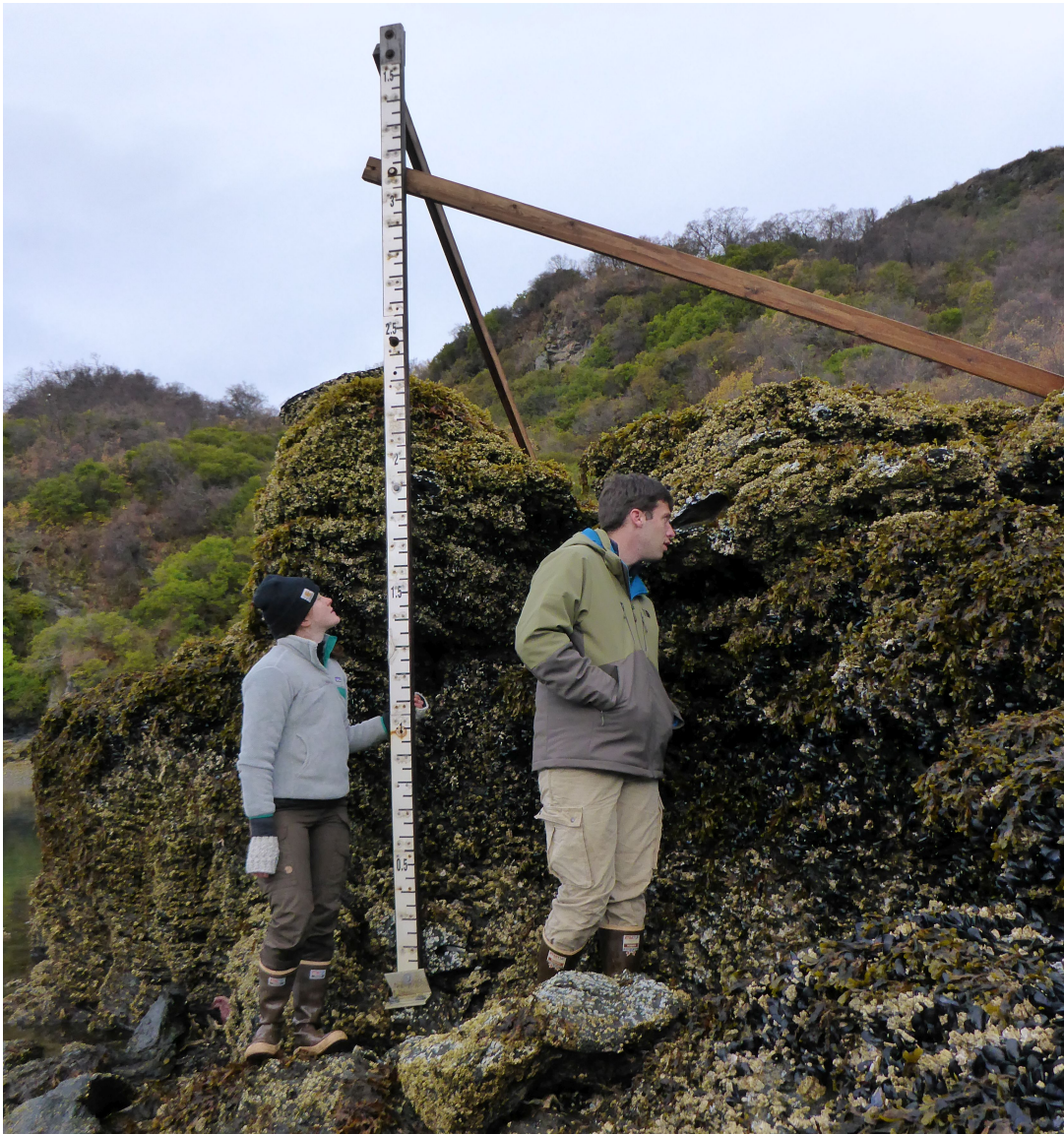
Figure 29: An example of a typical Rainier tide staff.
