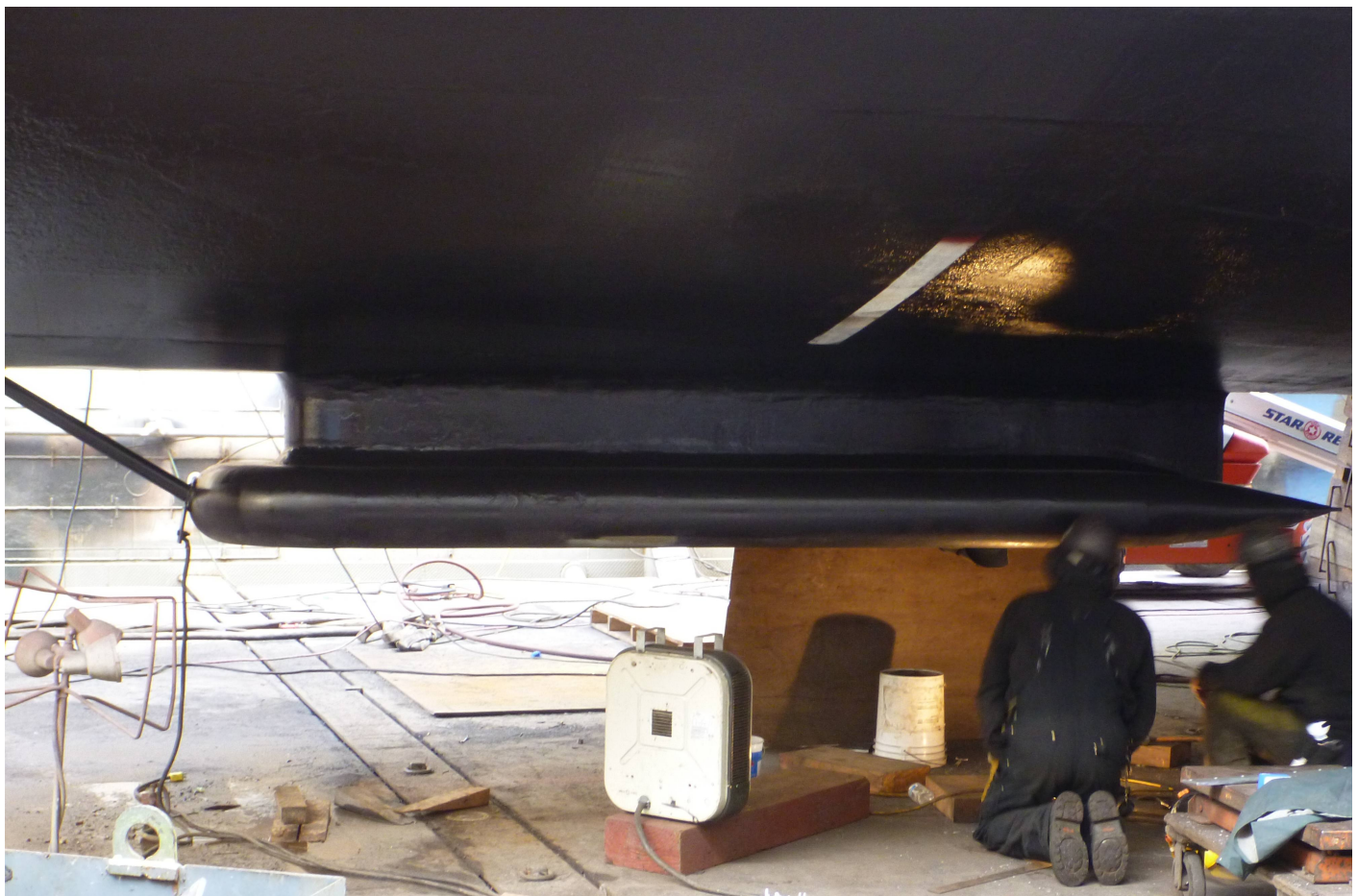
Figure 9: Kongsberg EM710 sonar transducer housing on Rainier (S221).
