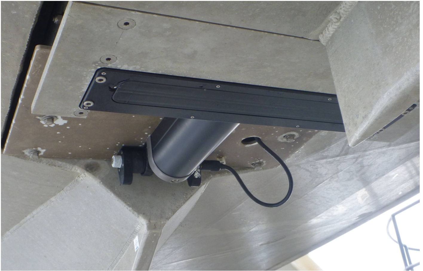
Figure 11: Reson SeaBat 7125 SV2 mounted on survey launch 2804.
