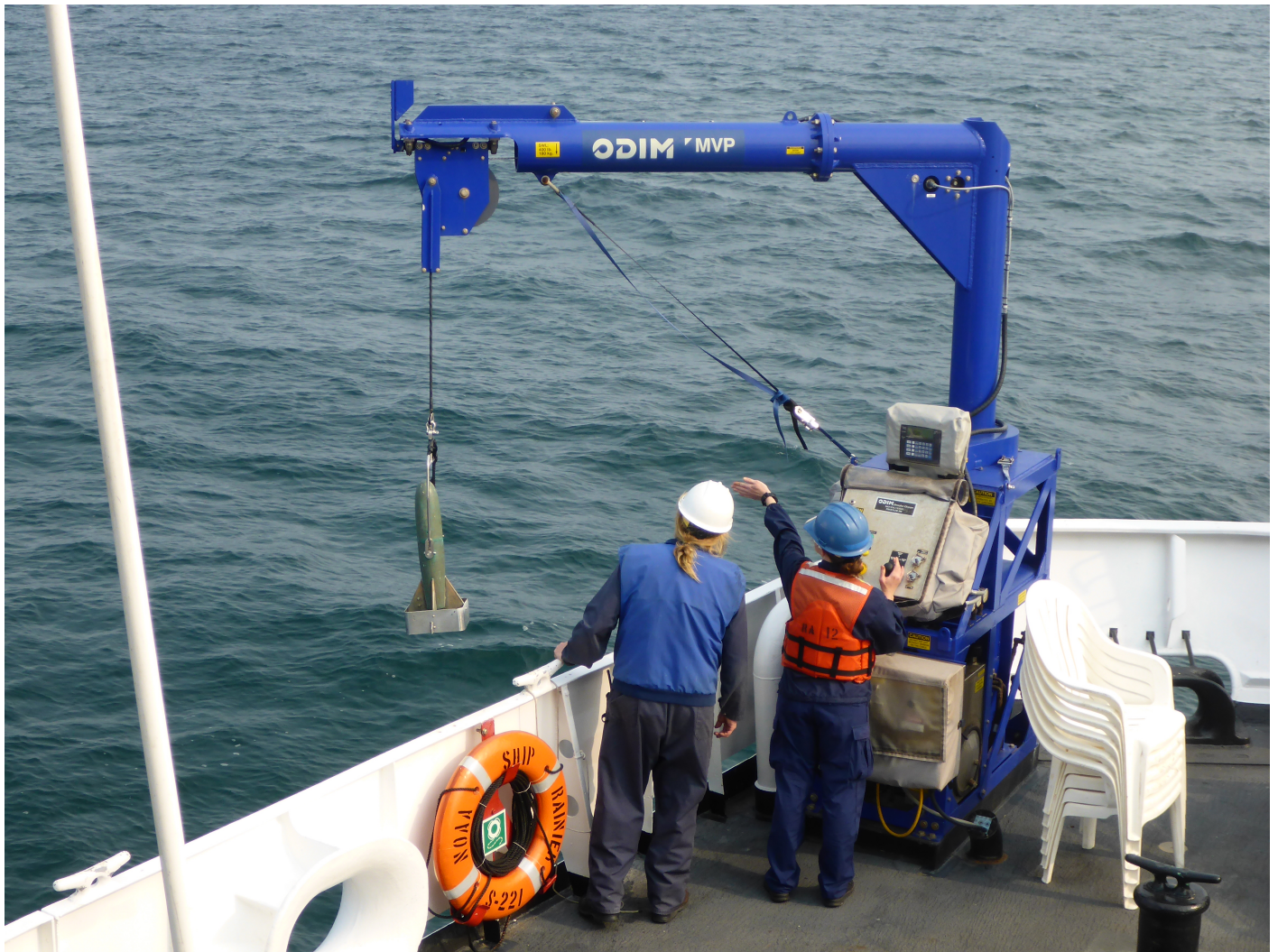
Figure 15: The ODIM Brooke Ocean MVP200 Moving Vessel Profiler being deployed from Rainier.
