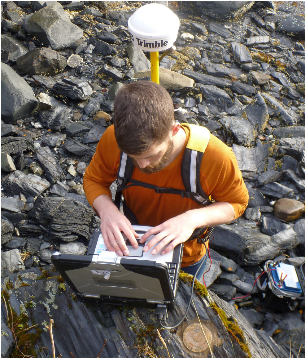
Figure 12: Trimble backpack GPS system connected to a Panasonic Toughbook laptop computer deployed to position benchmarks at a tide gauge installation.
