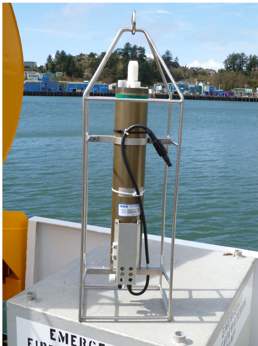
Figure 13: The SEACAT SBE 19 profiler. Note the band of electrical tape around the housing at the top of profiler marking this as the "green" CTD.
