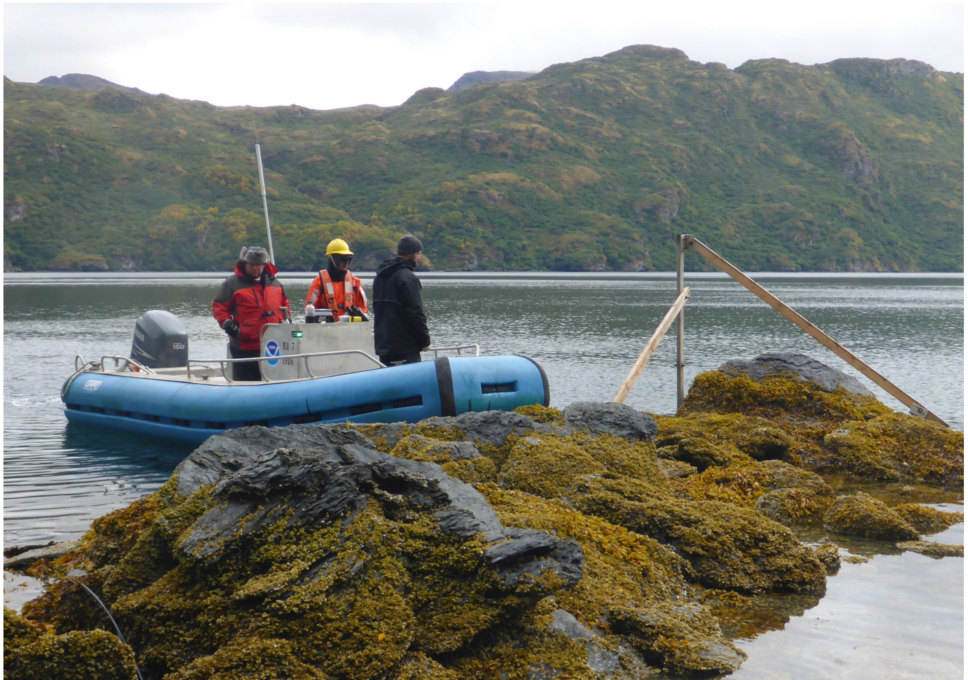
Figure 6: Rainier survey skiff RA7 (1906) conducting tide staff observations
