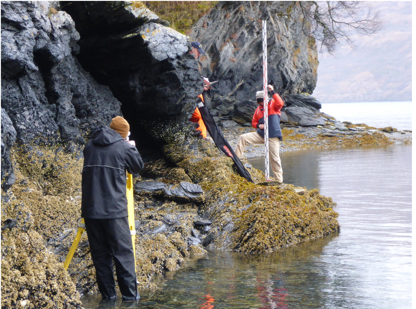
Figure 20: A Zeiss Ni2 optical level being used in the field.
