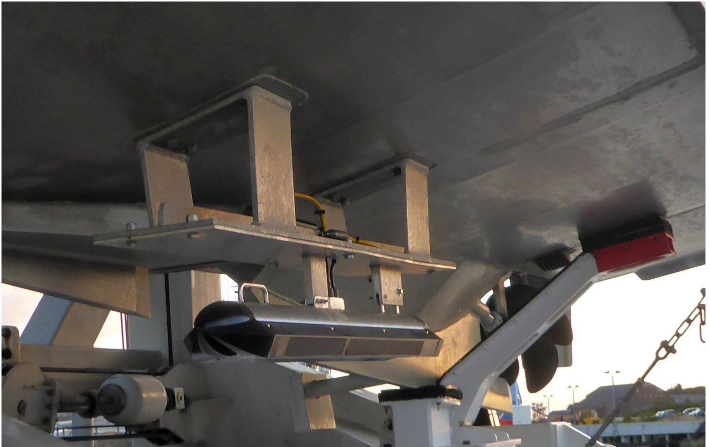
Figure 8: An Edgetech 4200 side scan sonar fish hull-mounted on 2804 (RA6).
