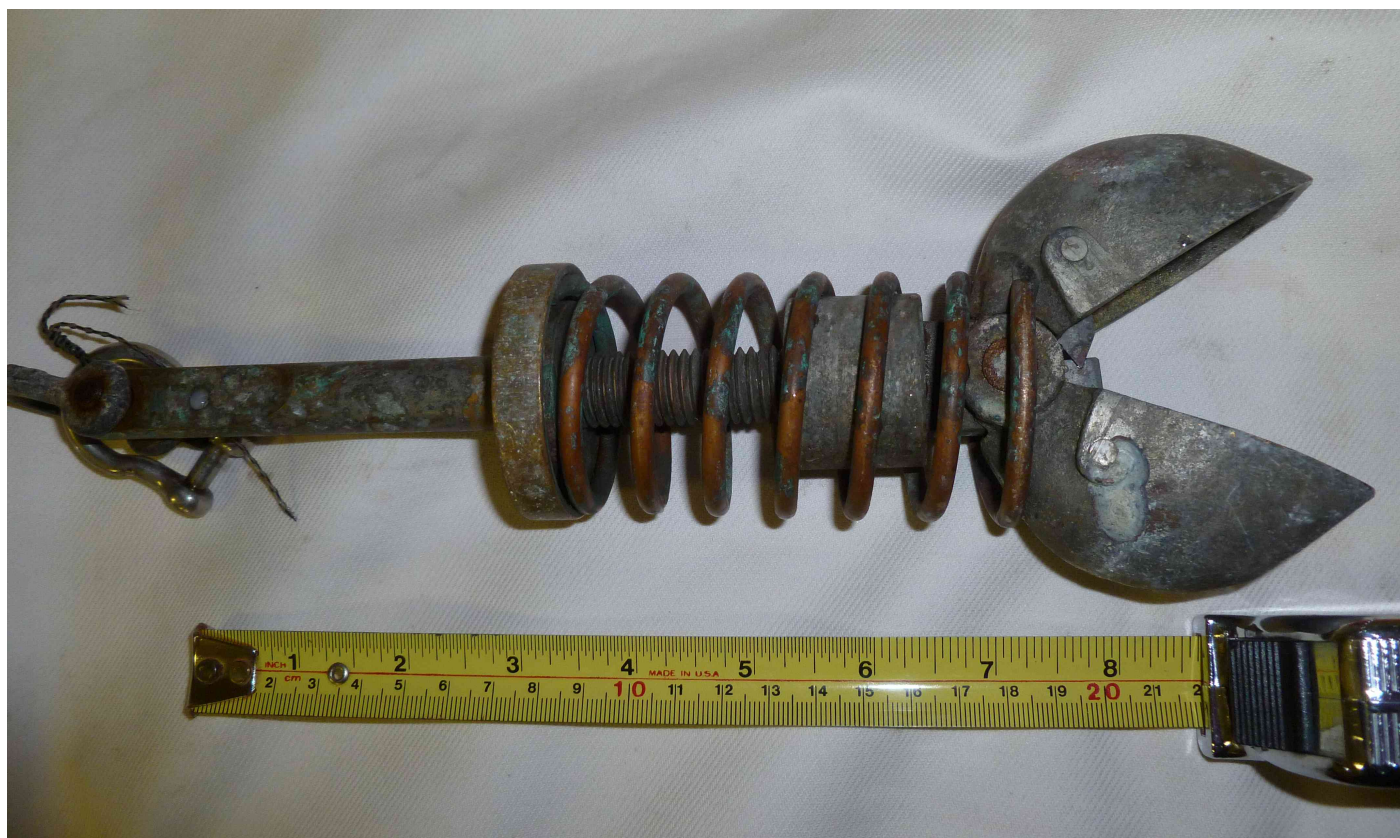
Figure 22: The “Nibbler” clam shell style bottom sampler.
