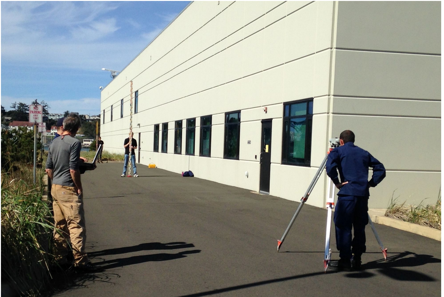
Figure 21: A preseason Kukkamaki test performed on a Zeiss Ni2 optical level at Pacific Marine Center, Newport Oregon.
