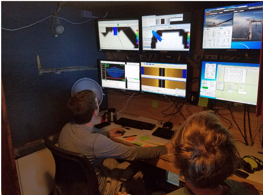
Figure 6 – Q105 data acquisition station, with direct interfaces to survey hardware.
