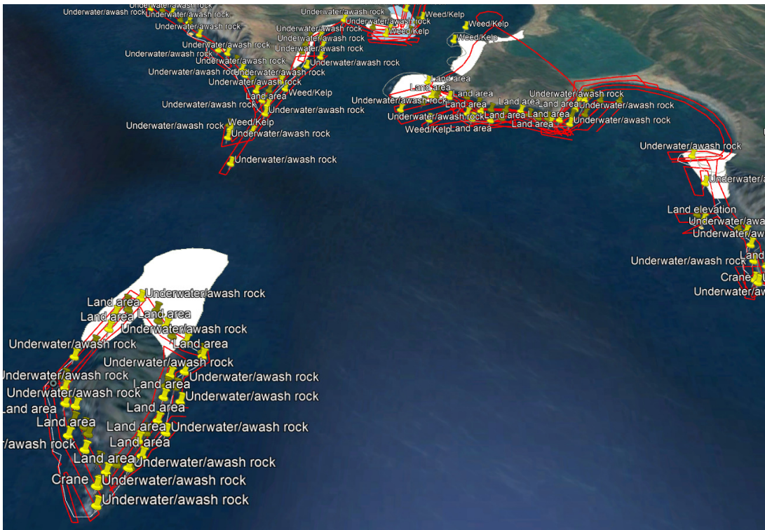
Figure 14 -- Pre-defined mission routes (red lines) over assigned features shown in Google Earth.
