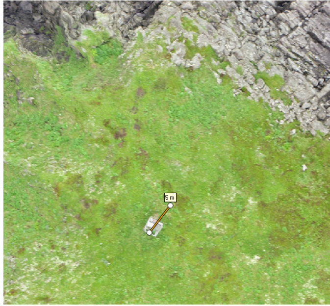
Figure 27 Mission 24 orthomosaic compared to charted Ikatan Point Light position, showing a 5 m horizontal difference.
