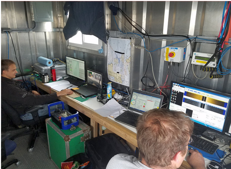
Figure 7 – Station aboard the Q105 for remotely controlling and monitoring the ASV-CW5. Displays are transmitted wirelessly from the unmanned vessel.
