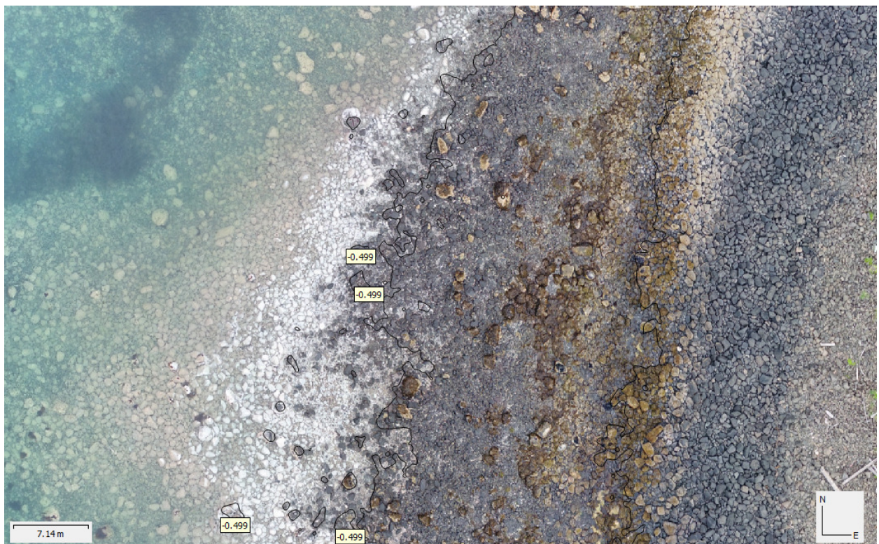
Figure 20 -- Waterline contour corrected for MLLW overlaid on DEM generated photo-mosaic in PhotoScan. A tide of -0.499 m at this mission time was assigned to the shoreline-water interface to adjust the final DEM to MLLW.
