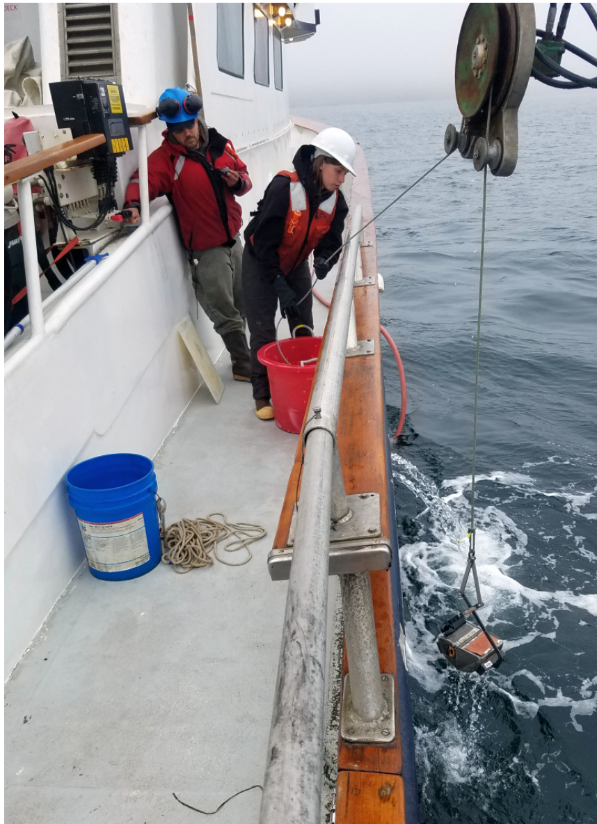
Figure 9 – Bottom sample collection with Van Veen sampler on the Q105 during this project.
