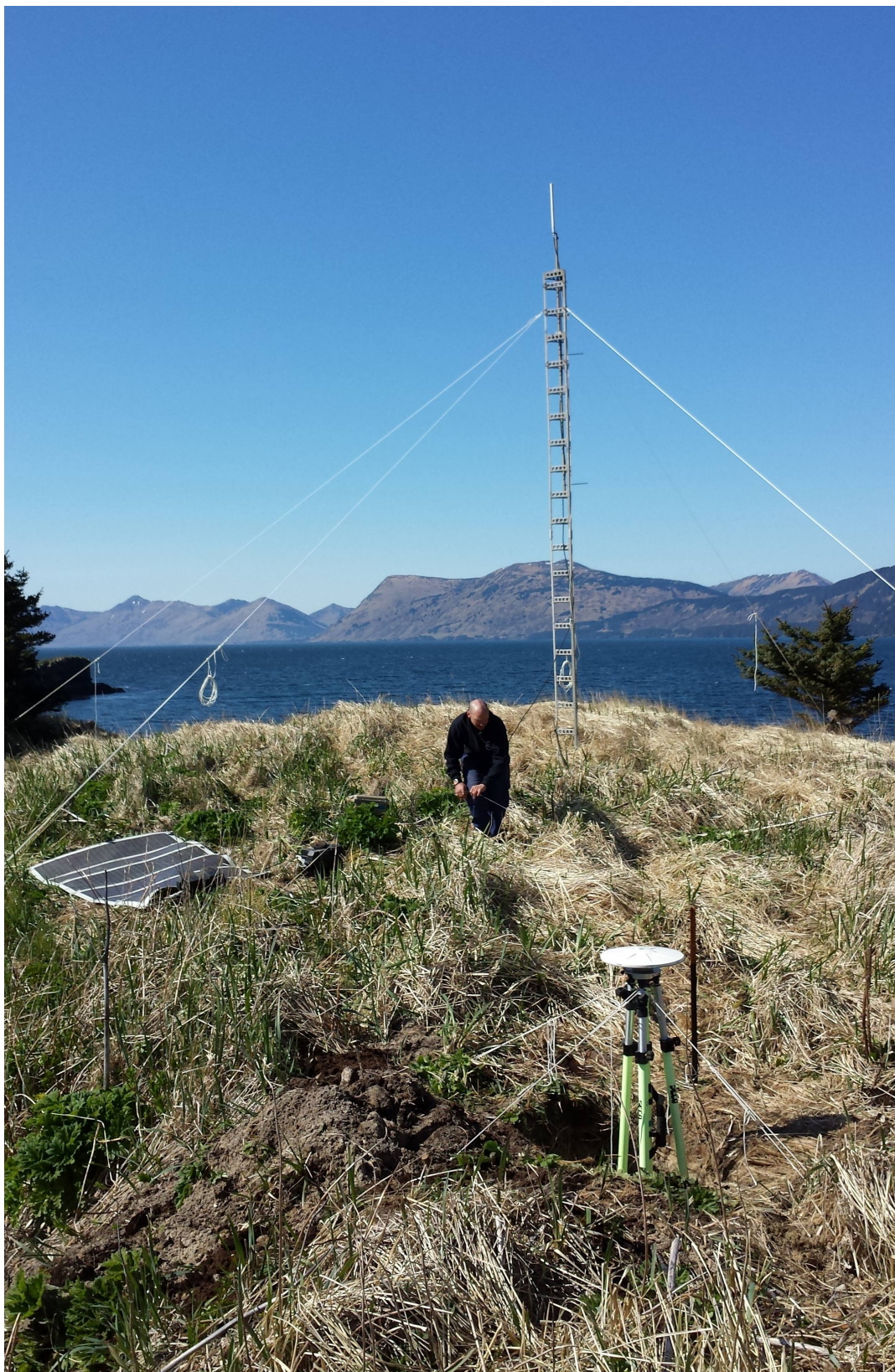
Figure 28: A Rainier base station installed in Kupreanof Strait, Kodiak Island, Alaska. Note the UHF antenna mounted on top of the 20 foot tower for extended range.
