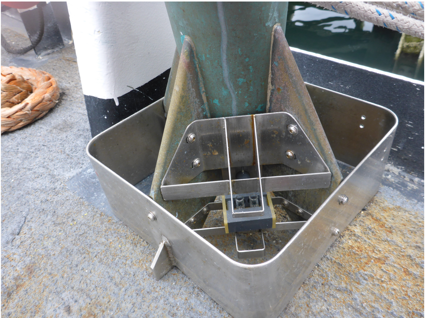
Figure 15: The stainless steel sensor guards as installed on the MVP200 fish.
