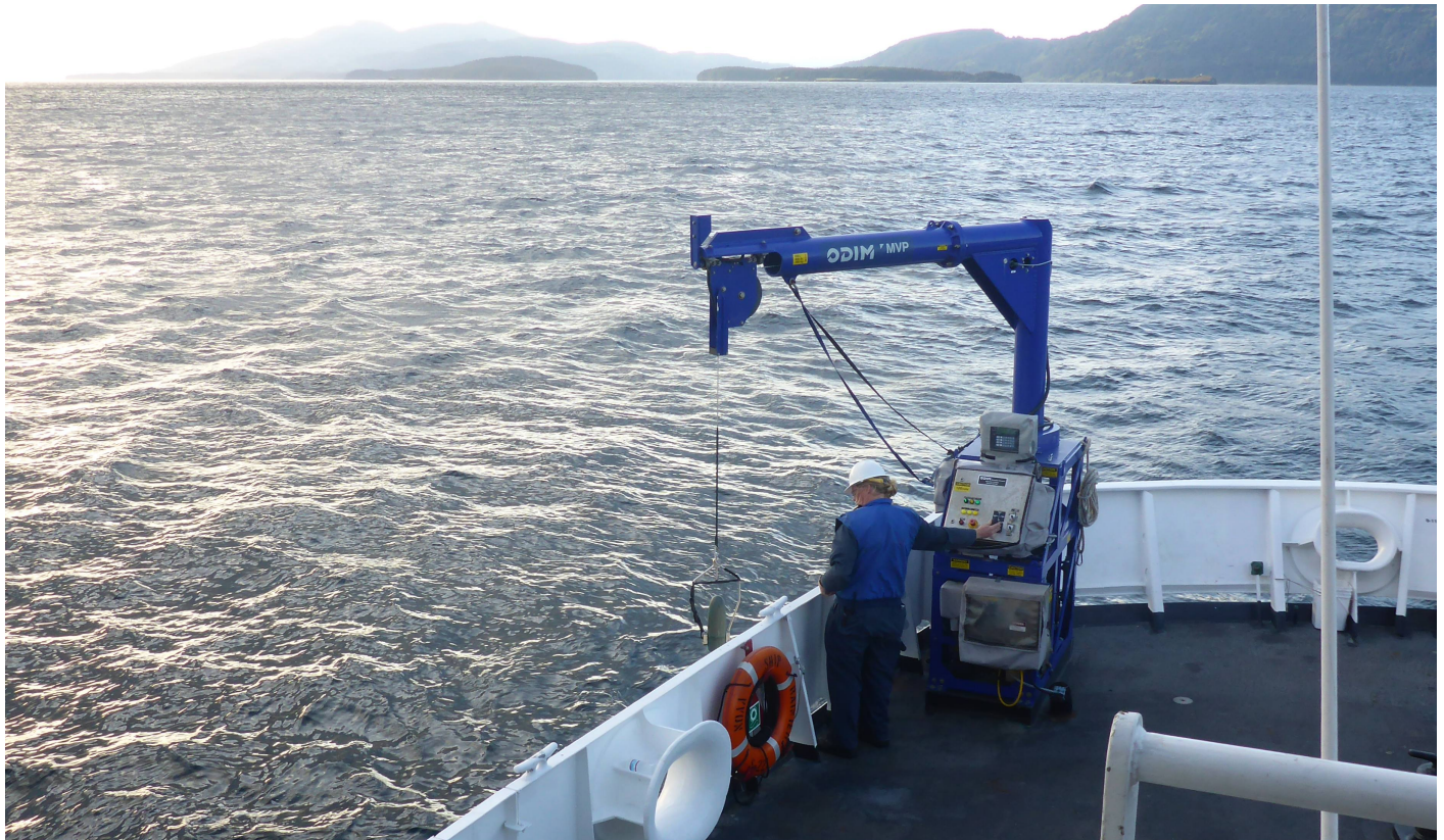
Figure 14: The ODIM Brooke Ocean MVP200 Moving Vessel Profiler being deployed from Rainier.
