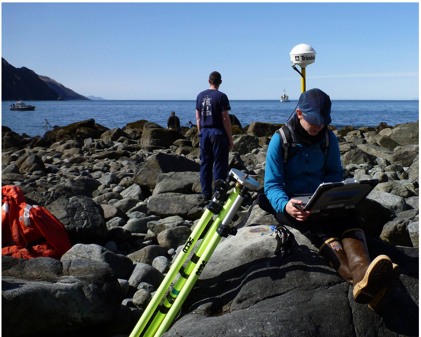
Figure 11: Trimble backpack GPS system deployed to position benchmarks at a tide gauge installation.
