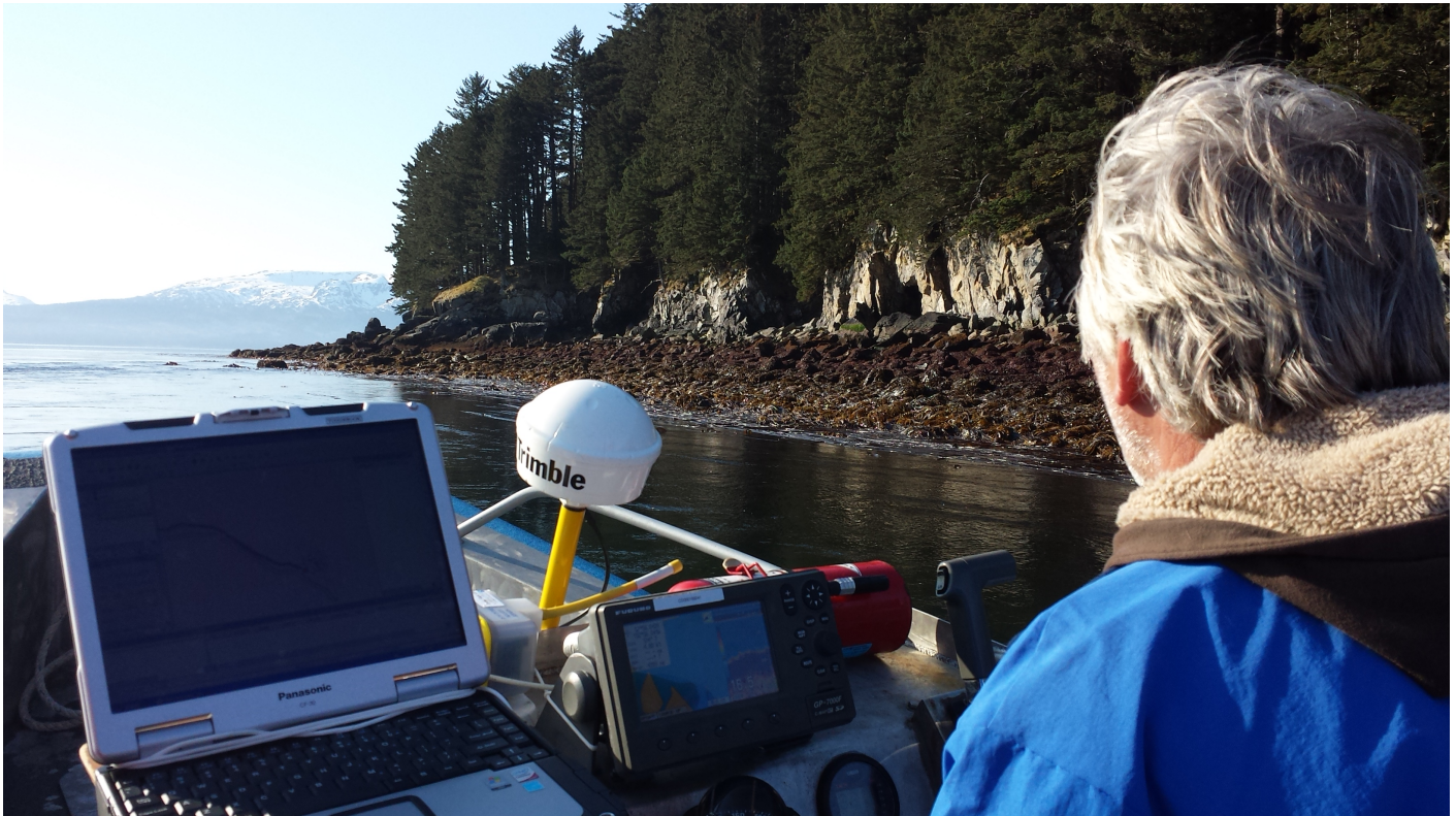
Figure 31: Survey skiff RA7 collecting the along-shore buffer line using a Trimble GPS backpack system connected to a Toughbook computer.
