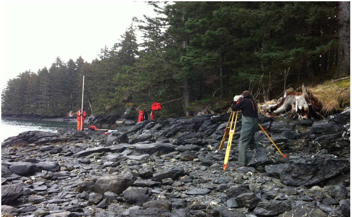
Figure 20: A Zeiss Ni2 optical level being used in the field.
