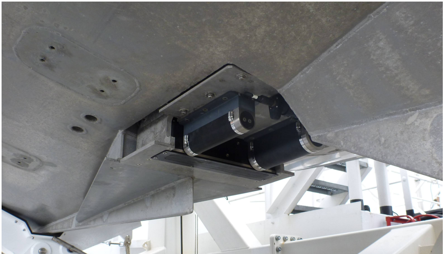
Figure 9: Reson SeaBat 7125-B mounted on survey launch 2801.
