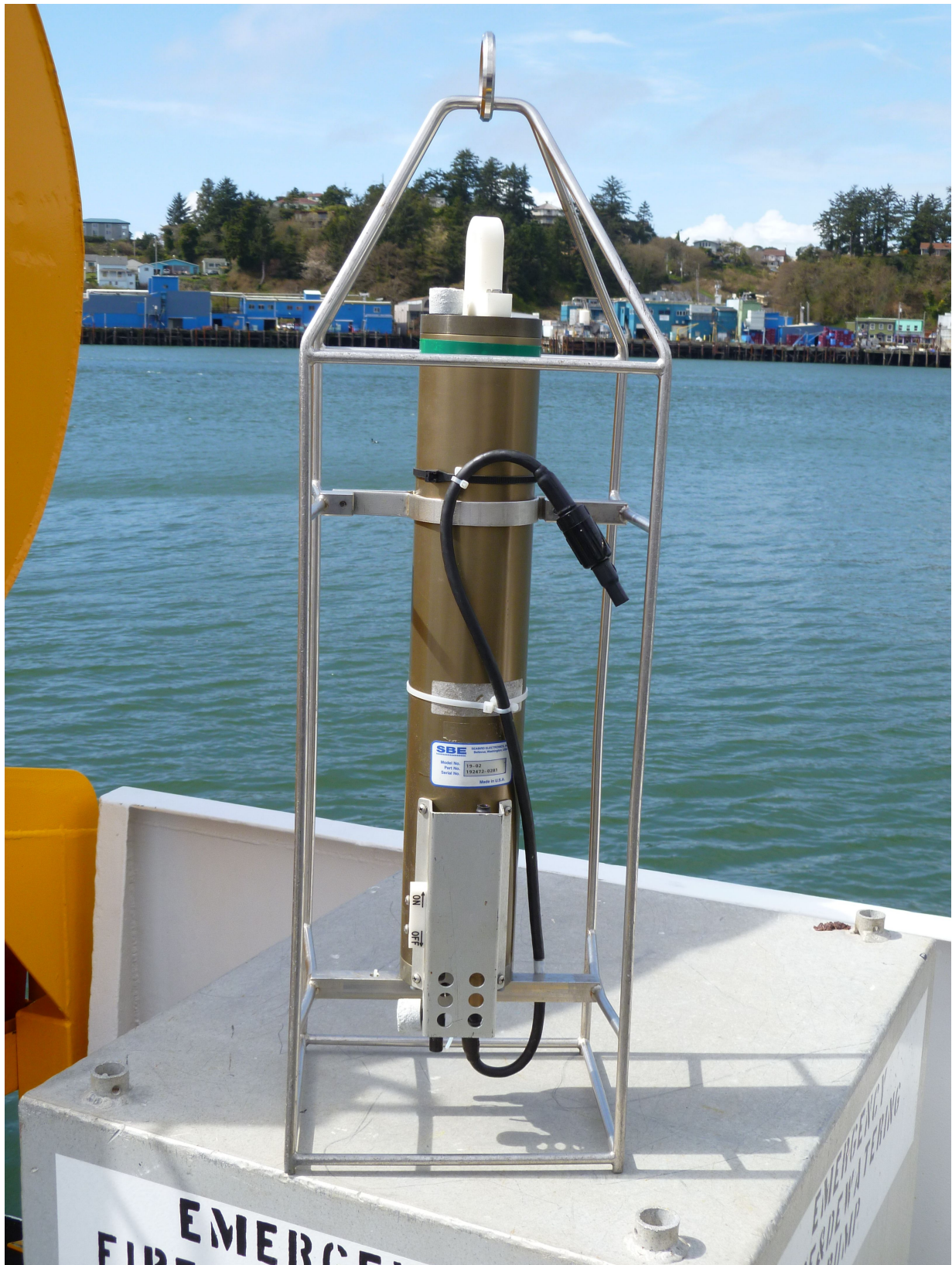
Figure 12: The SEACAT SBE 19 profiler. Note the band of electrical tape around the housing at the top of profiler marking this as the "green" CTD.
