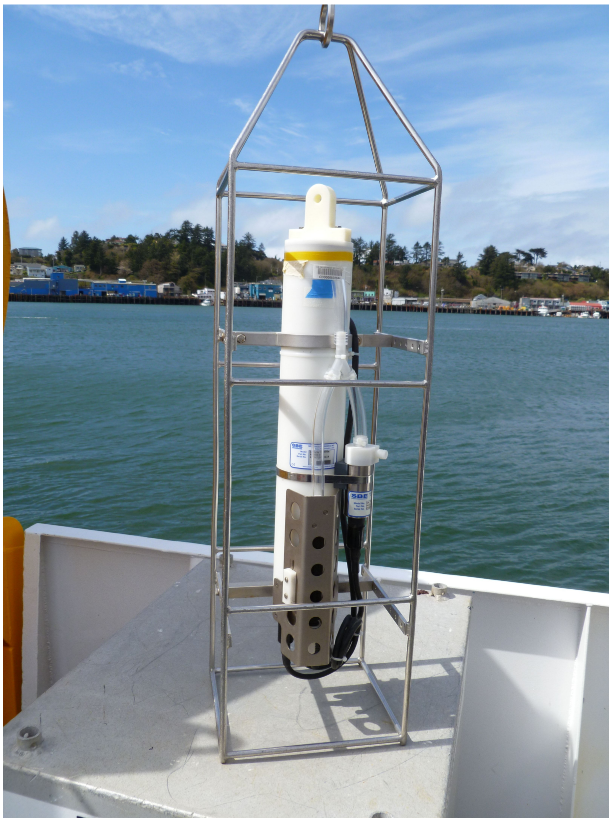
Figure 13: The SBE 19plus SEACAT profiler. Note the band of electrical tape around the housing at the top of profiler marking this as the "yellow" CTD
