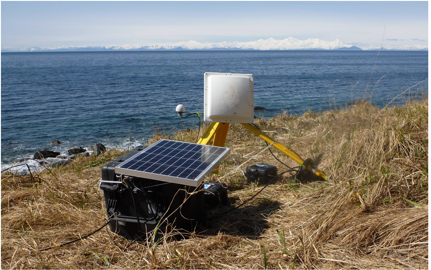
Figure 29: A Portable Tide Gauge (PTG) system with GOES and GPS antennae mounted on an aluminum tripod and a solar panel secured to the top of the gauge case.
