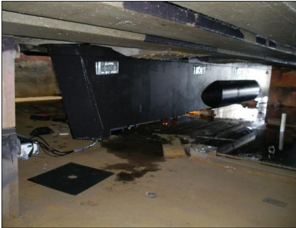
Figure 9 M/V Ocean Pioneer Drop Keel with 7125
