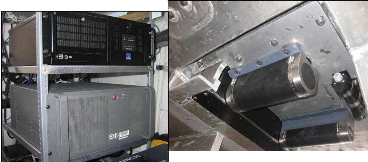
Figure 5: Reson 7125SV on a Fairweather Launch
