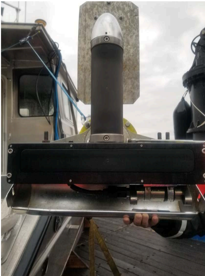
Figure 3: MBES mounting configuration shown on Skiff
