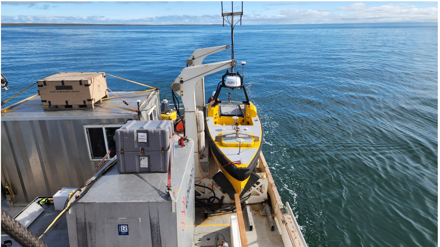
Figure 2: The ASV-CW5 in its launch system on the back deck of the Q105.
