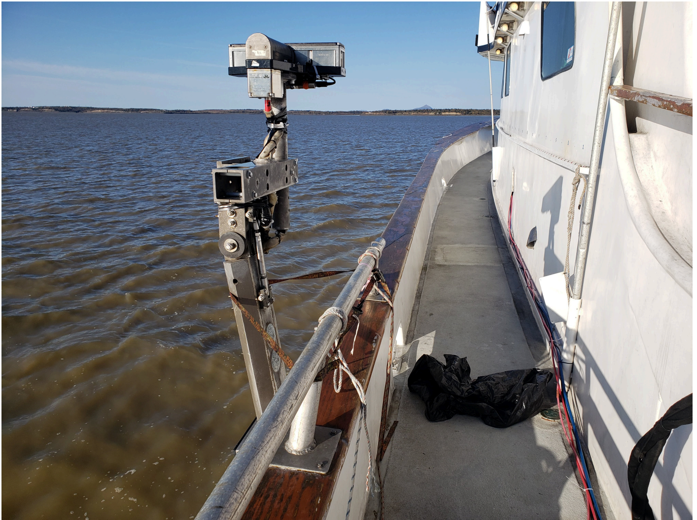
Figure 4: T50 mounted on hydraulic arm on the Q105.
