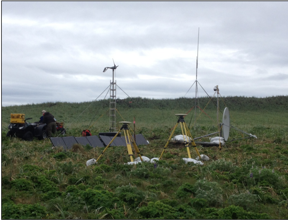
Figure 5 – Cape Chunak base station. NetRS (left) and T5700 (right) GPS antennas in foreground.
