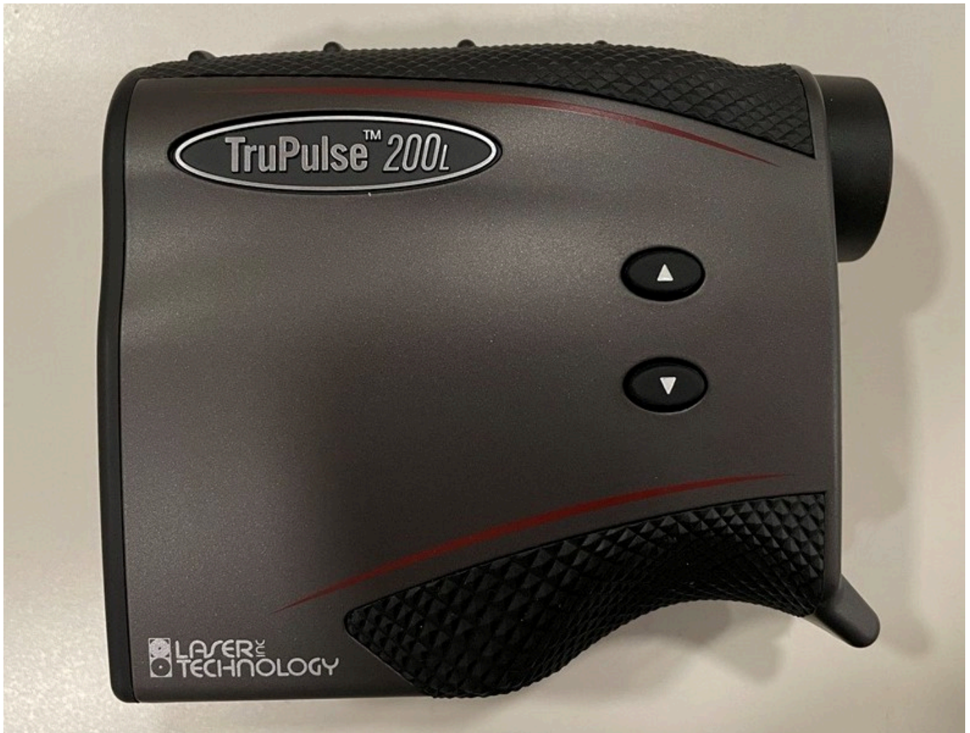
Figure 21: Laser Technology TruPulse 200L Laser Range Finder
