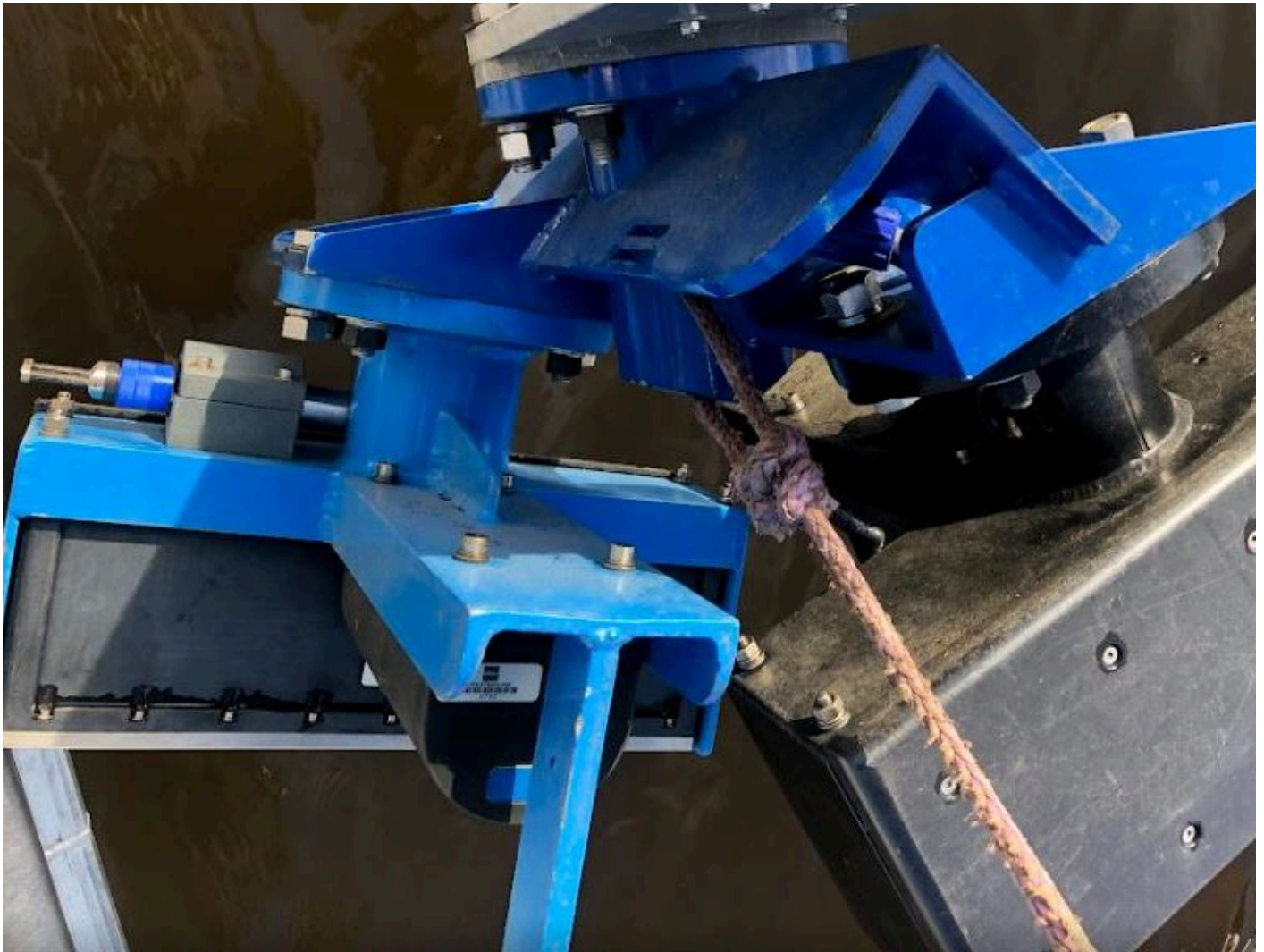
Figure 14: AML Micro•X installed on a dual head R2Sonic 2024 custom mount
