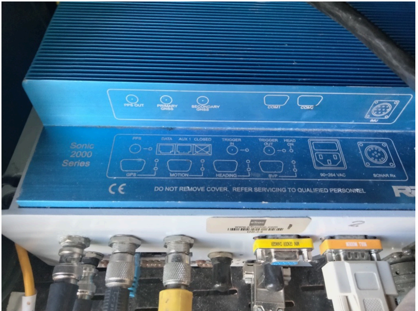
Figure 11: I2NS Sonar Interface Module (SIM)
