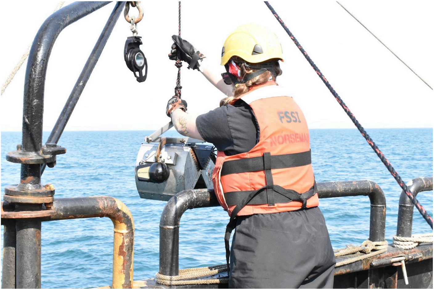
Figure 22: Ponar Grab in use for bottom sample collection
