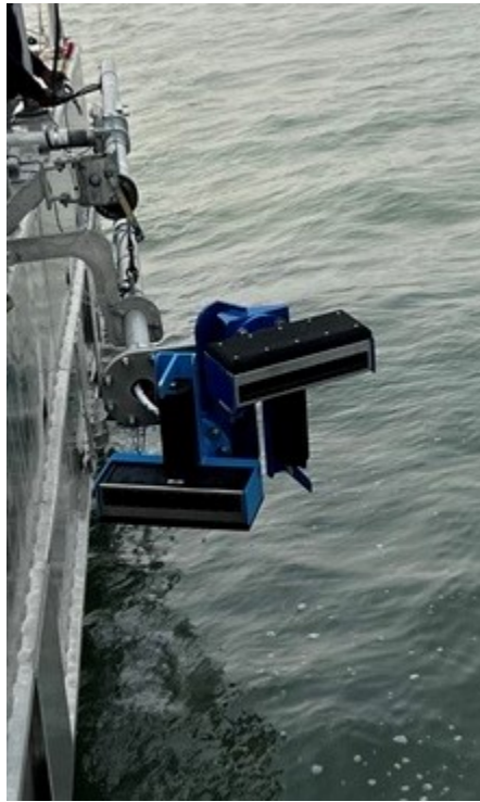
Figure 6: R2Sonic 2024 MBES (dual head)
