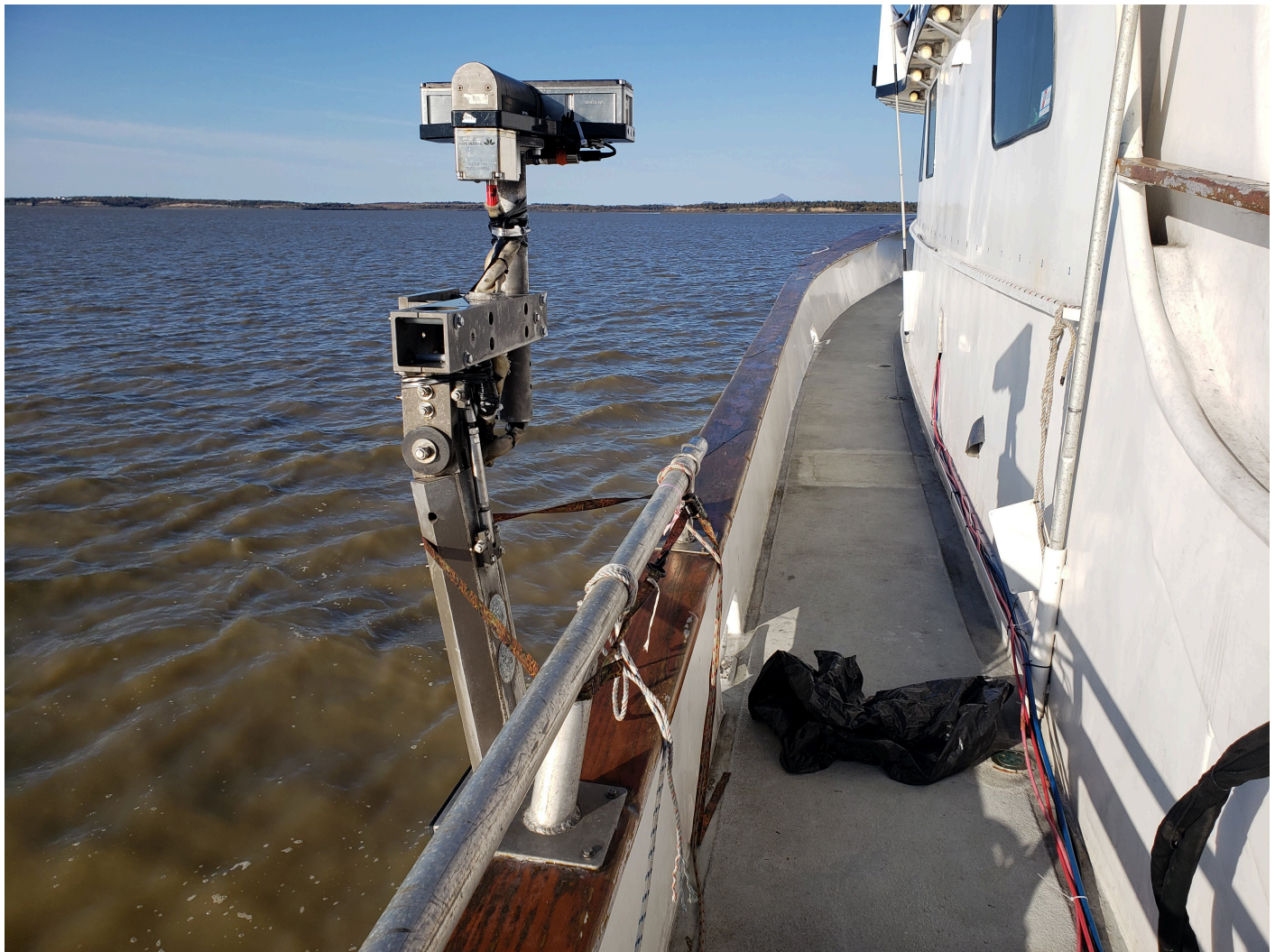
Figure 3: Teledyne Reson SeaBat T50-R transducer mounted on Q105's hydraulic arm in up position.
