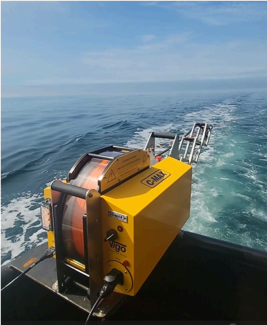
Figure 9: Vigo Winch mounted on the Arctic Seal starboard stern.
