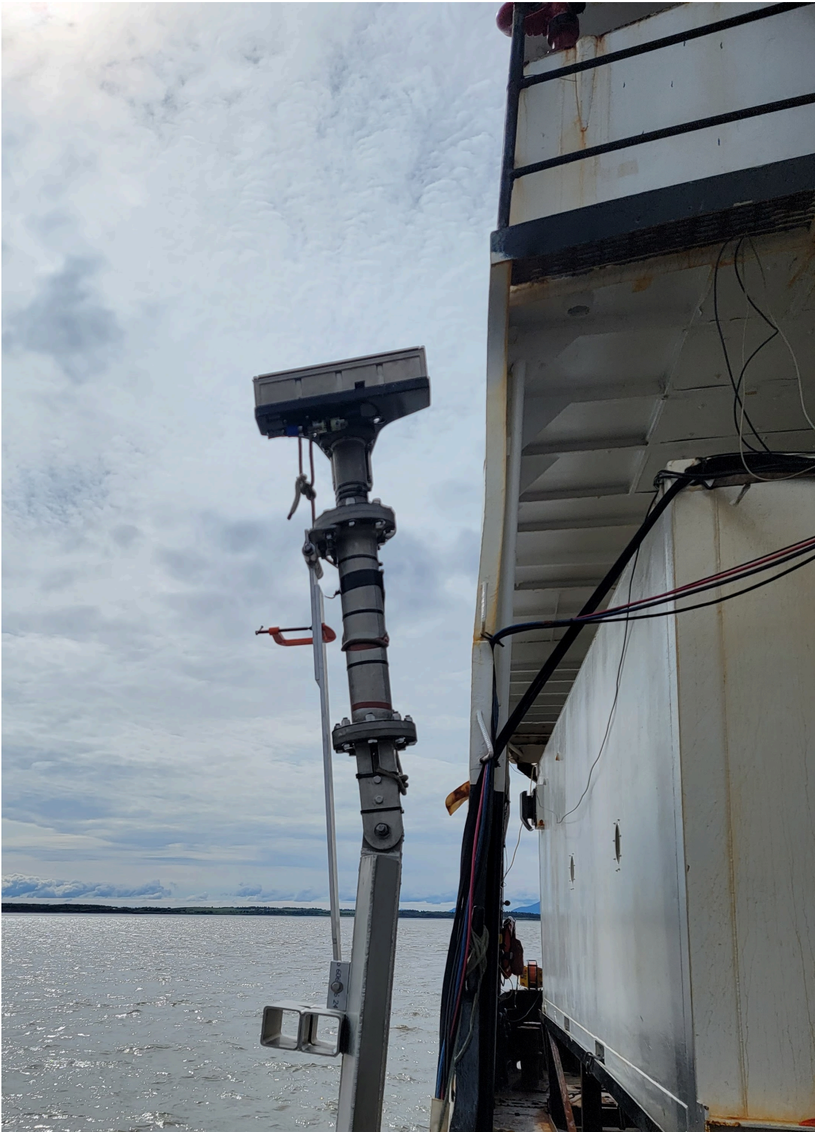
Figure 5: T50-R mounted on the Arctic Seal's Hydraulic Arm.
