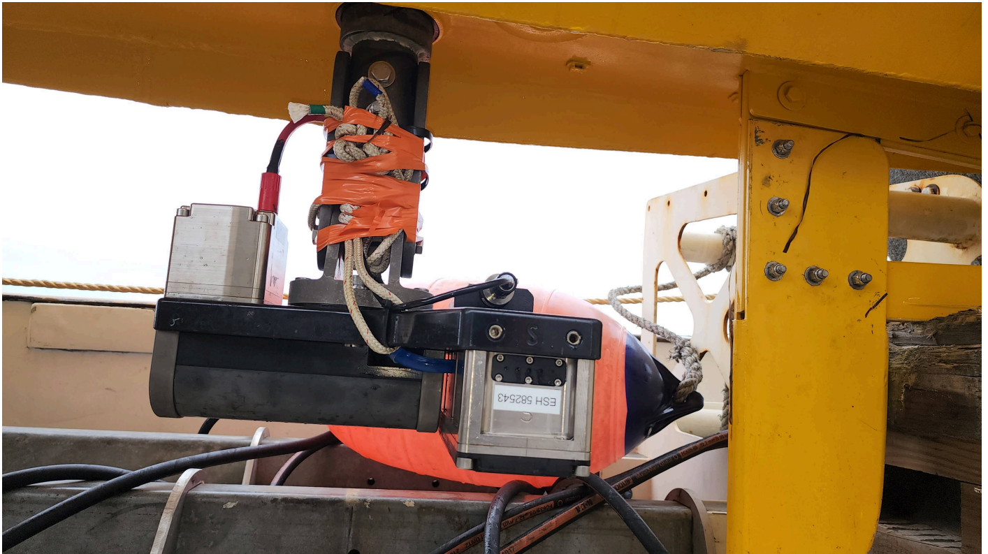
Figure 6: T50-R mounted on the ASV keel.
