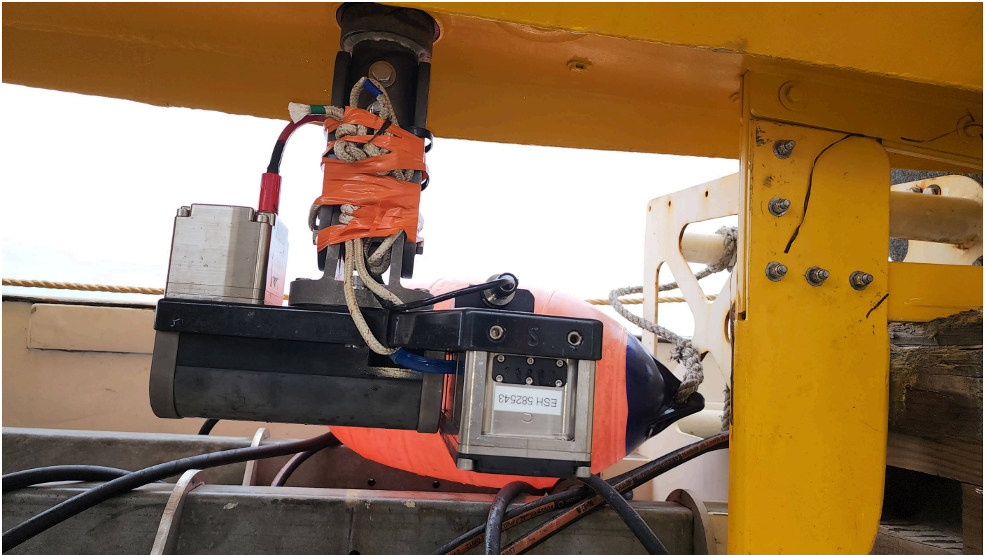
Figure 8: Applanix IMU-30 co-located on the ASV T-50 mounting bracket.
