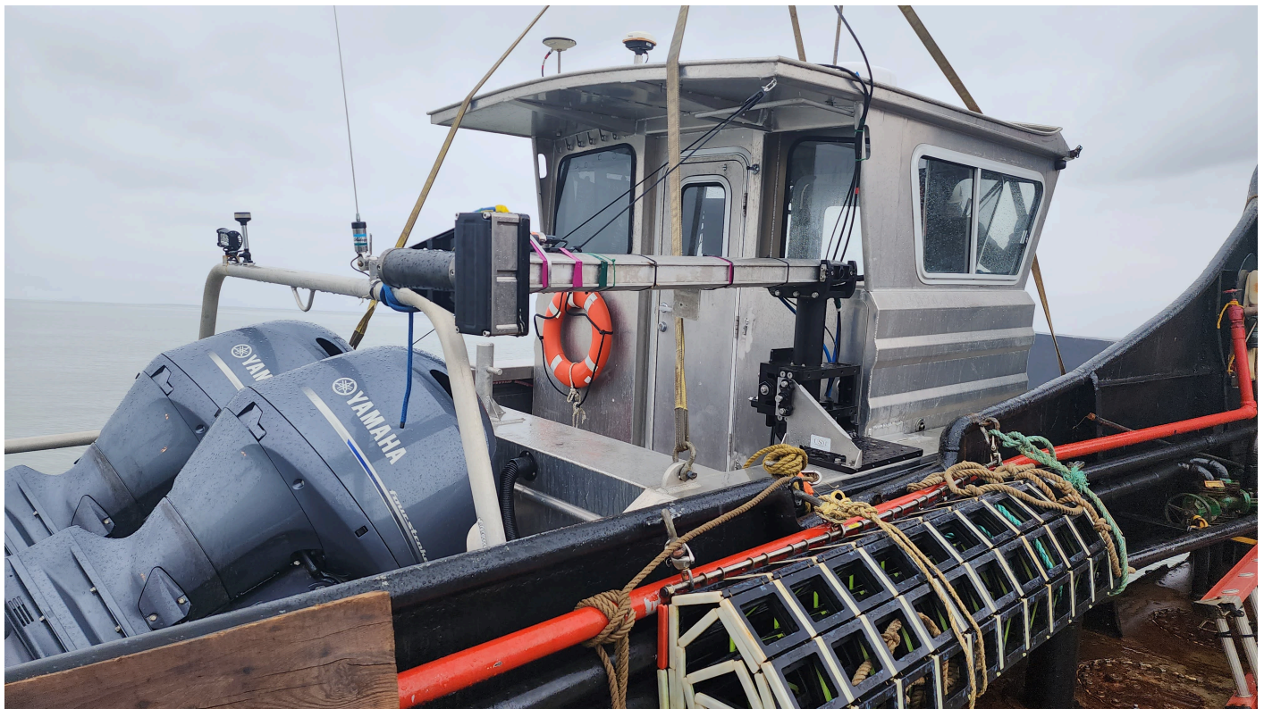
Figure 7: T20-P Mounted on LC-25 swivel pole.
