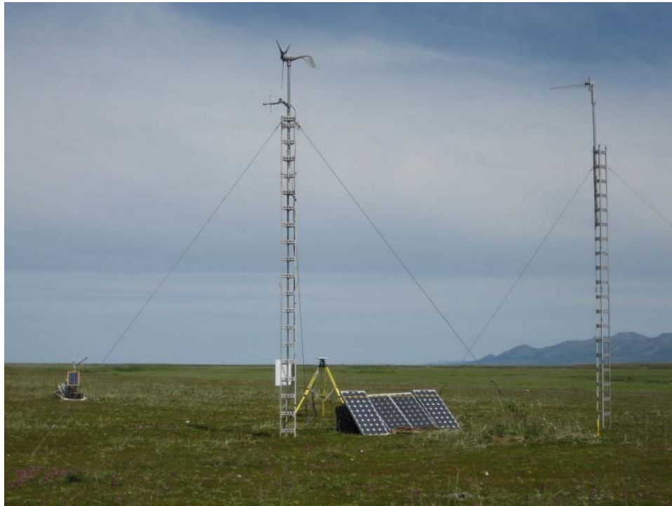
Figure 5 – RTK/PPK Base Station at Carter Bay
