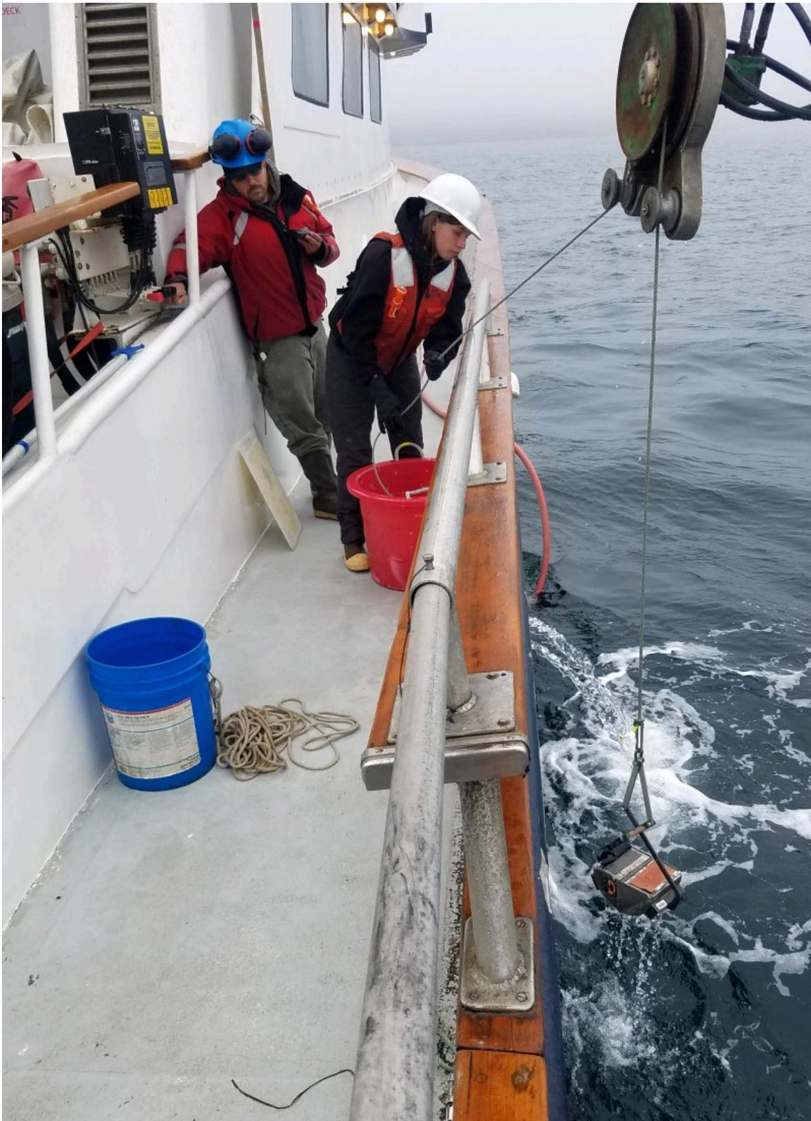
*Figure 9: Bottom sample collection with the Van Veen sampler on the Q105.*
