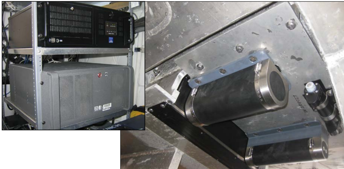
Figure 5: Reson 7125SV on a Fairweather Launch
