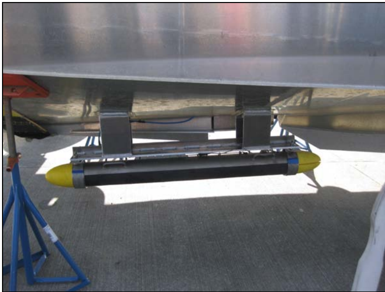
Figure 6: Hull-Mounted Klein 5000 Side Scan Sonar on Fairweather Launch
