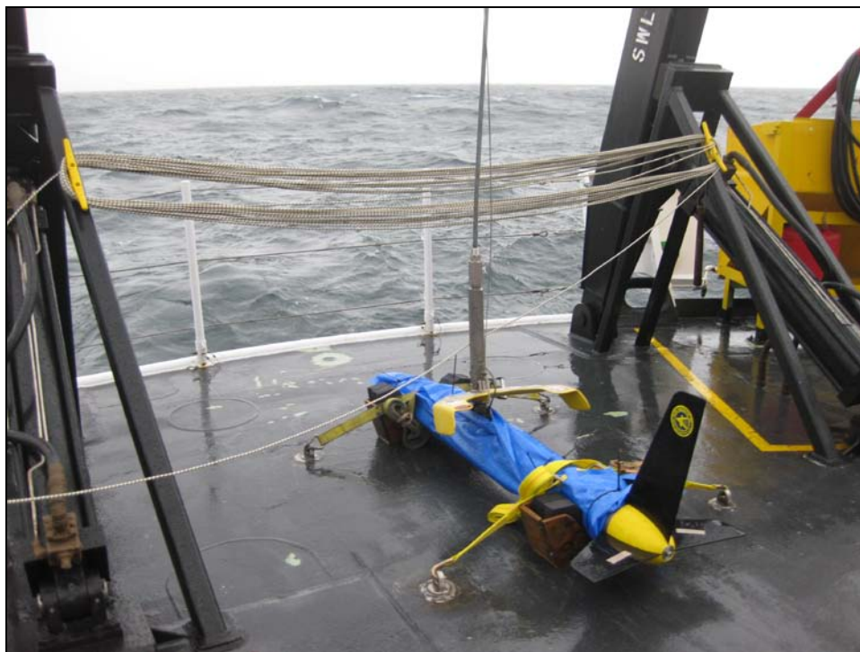
Figure 7: Towed Klein 5000 Side Scan Sonar on Fairweather
