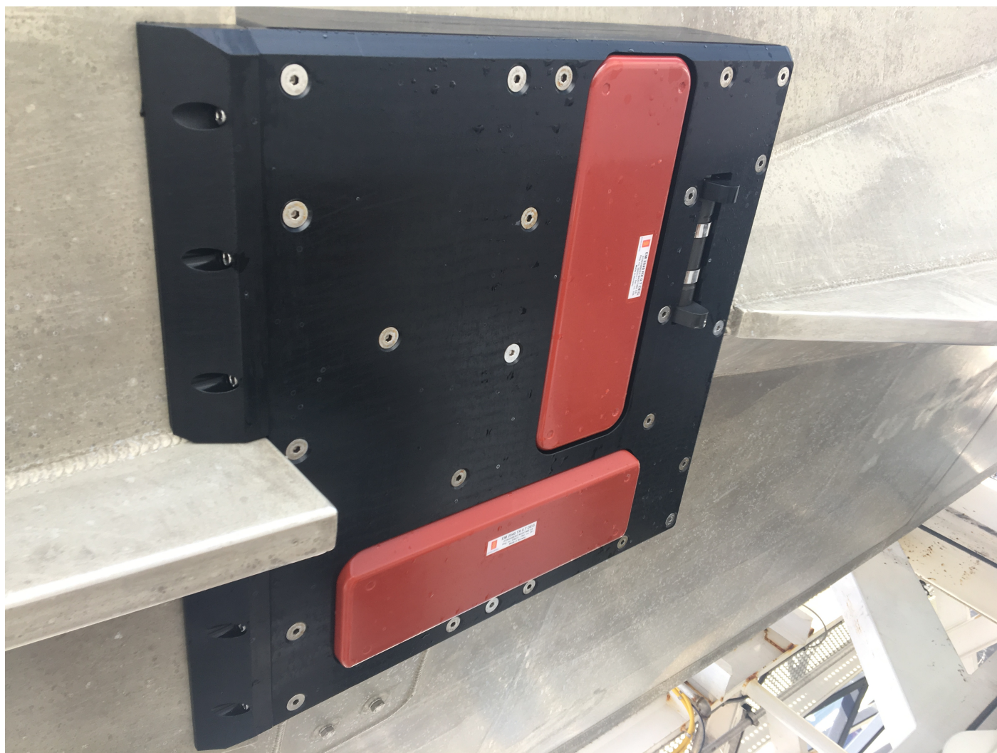
Figure 12: Kongsberg EM 2040 projector and receiver arrays
