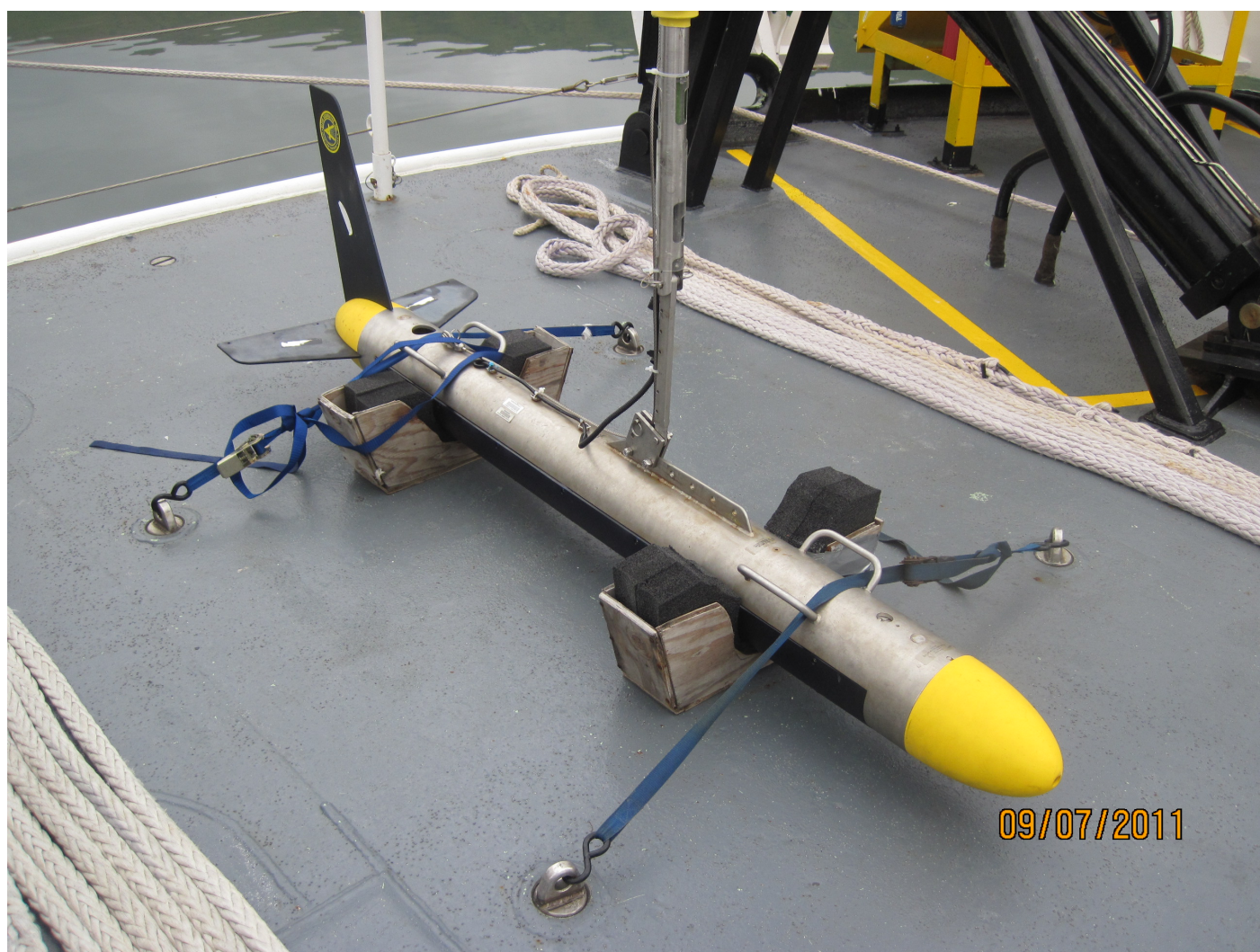
Figure 8: Towed Heavy Weight Klein 5000 Side Scan Sonar
