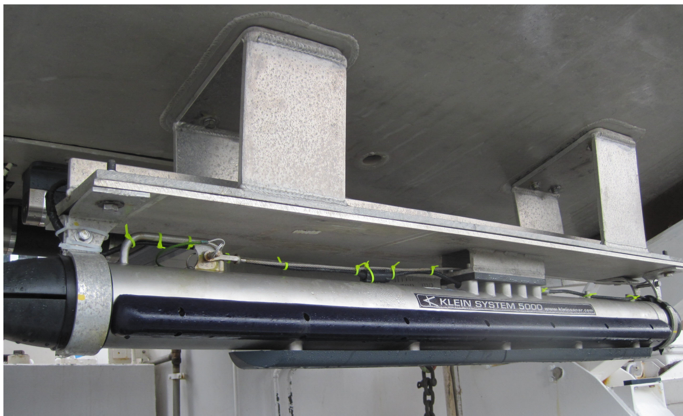
Figure 10: Hull-Mounted Light Weight Klein 5000 Side Scan Sonar
