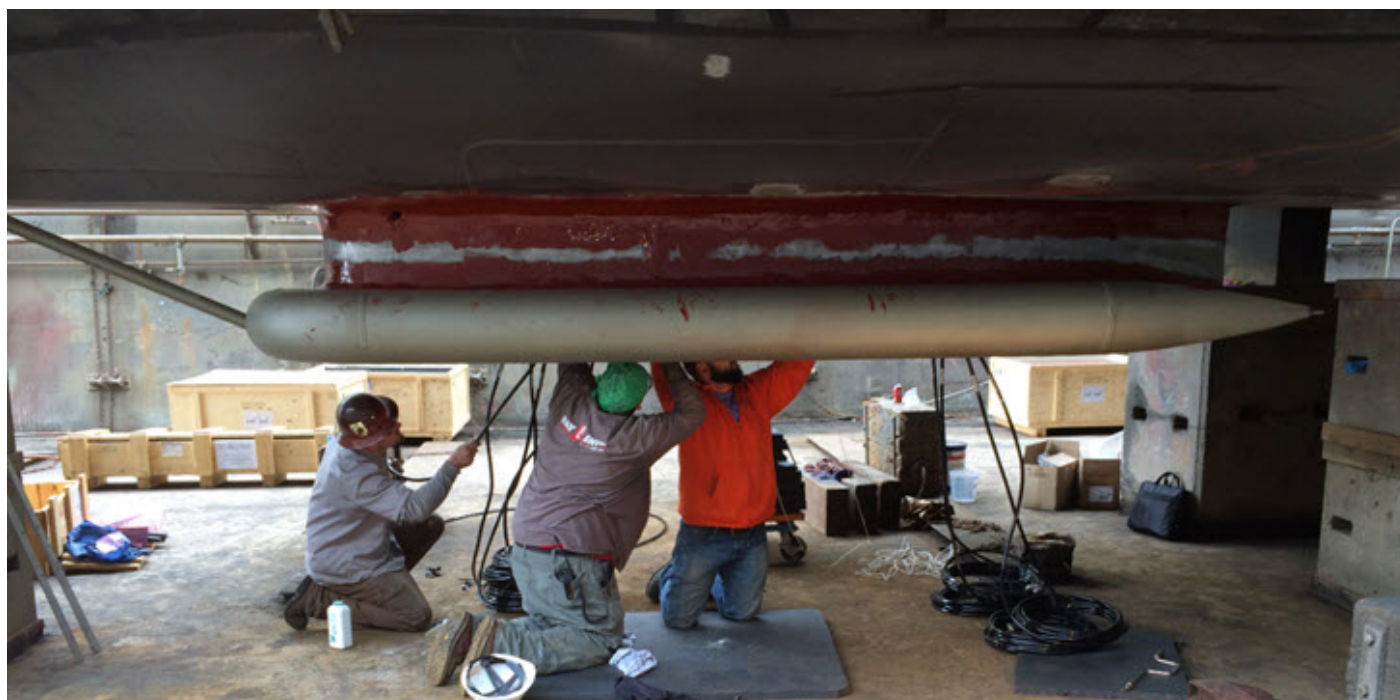
Figure 13: EM 710 Gondola during transducer installation.
