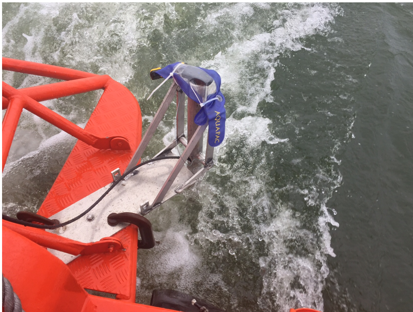
Figure 39: CEEPulse with submerged transducer on its pole mount
