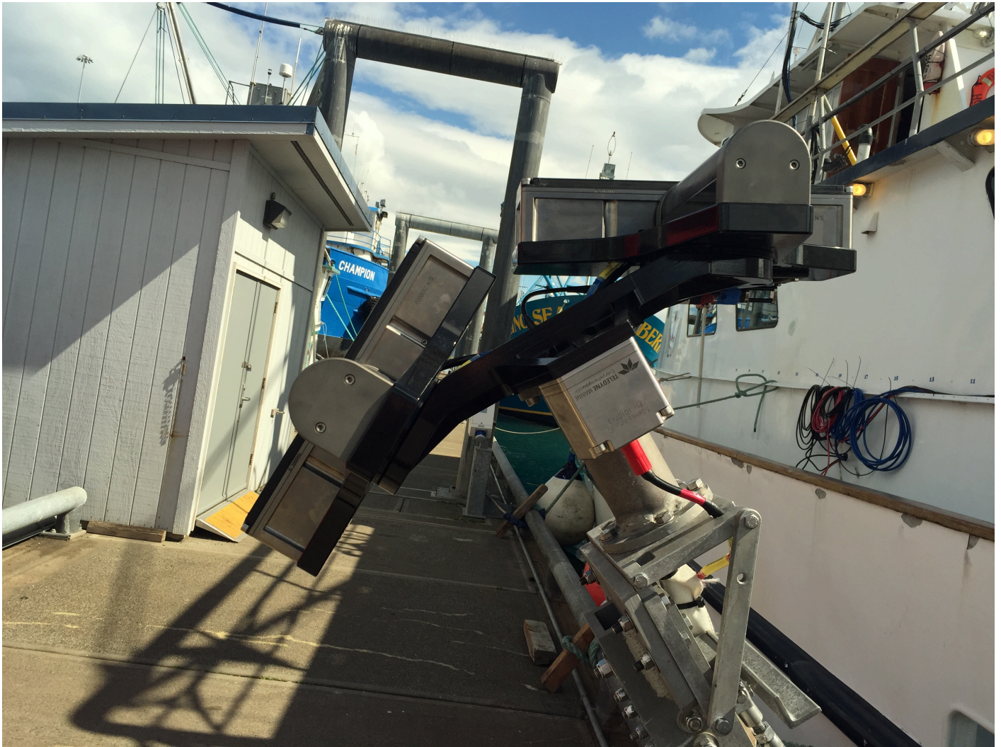
Figure 3: Teledyne Reson SeaBat T50-R IDH configuration mounted on Q105's hydraulic arm.
