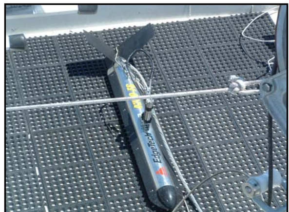
Figure 4. Edgetech 4200-FS Side Scan Sonar
