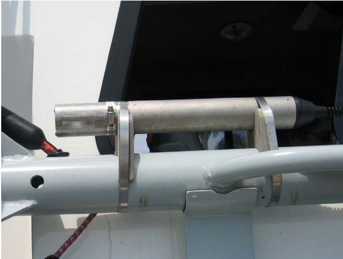
ODOM Hydrographic Systems Digibar Pro on Survey Launch S3003
