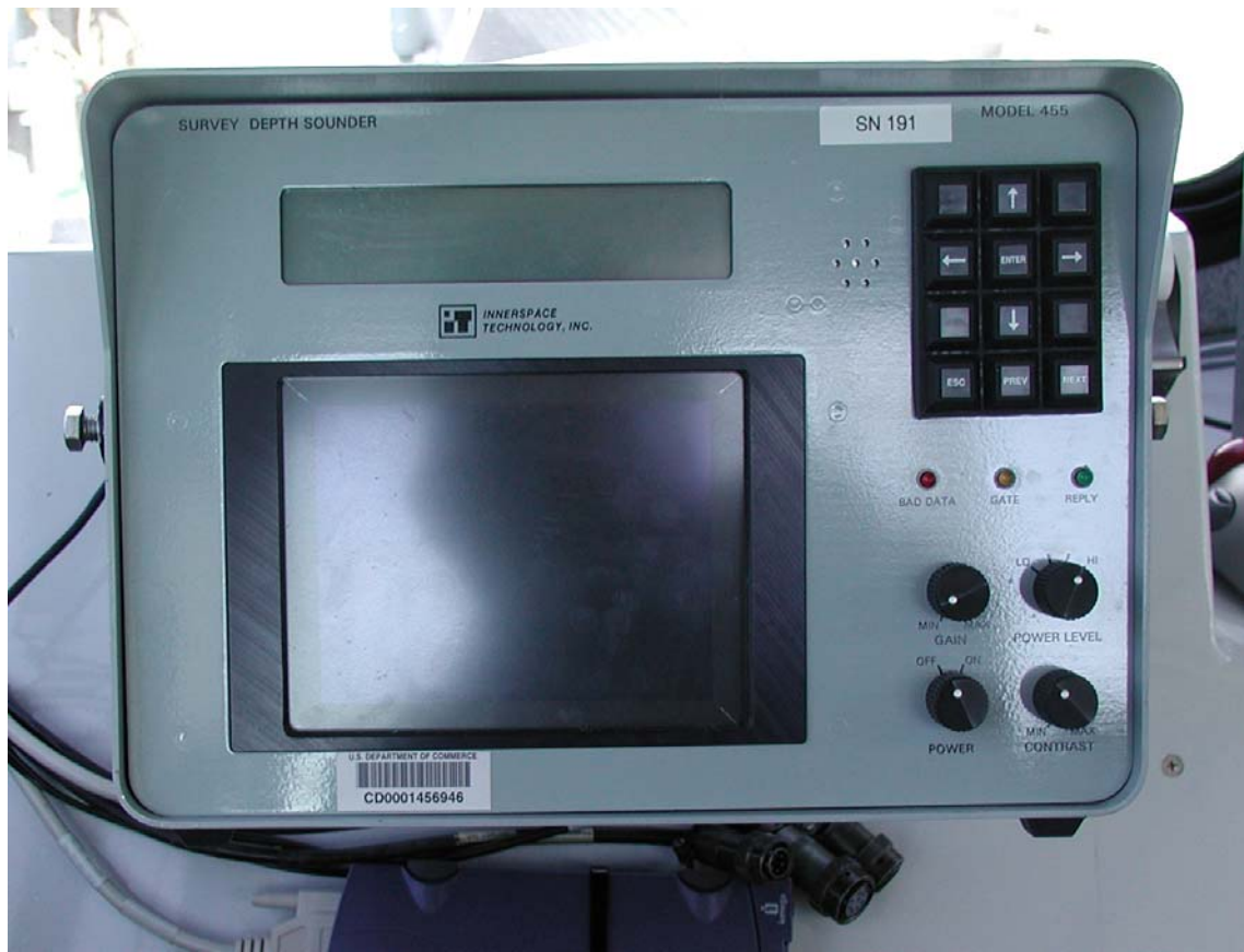
Innerspace Technology 455 Survey Depth Sounder on S3003
