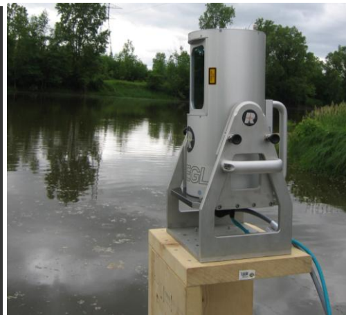
Laser Scanner installed on TtEC Jet Boat
