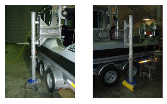
The Reson 8125 forms 240 beams each of which has a  $0.5^{\circ}$  across-track beam footprint for a maximum total swath width of 120°. Each beam has an along-track resolution of 1°. The ping rate is nominally 20-40 Hz, but may vary according to operating conditions. The Reson 8125 sonar is capable of bottom detection in depths from 3-120m. Specifications for this sonar are included in Appendix I of this report.
