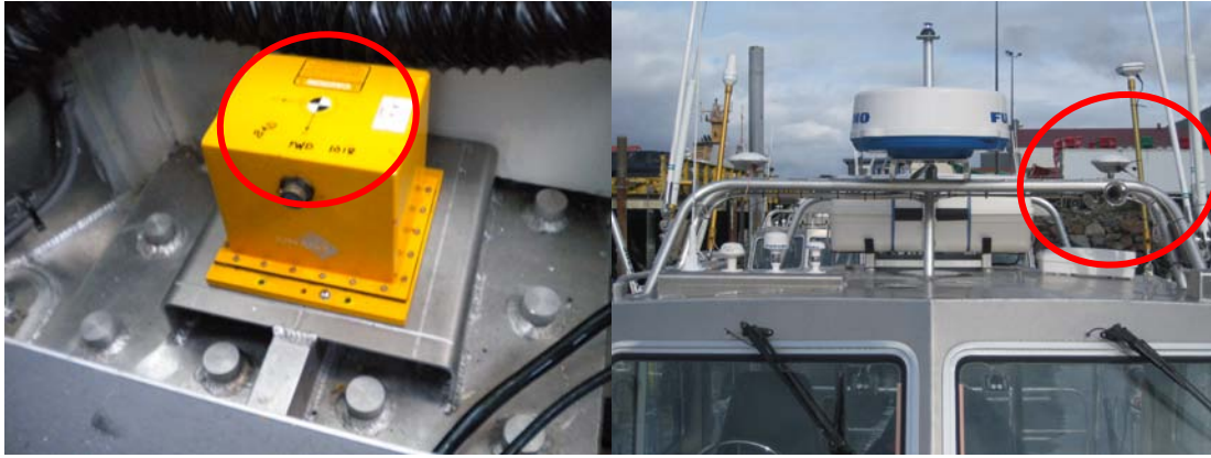
Figure 15: Vessel Reference Point (Center of POS/MV IMU) and Primary GNSS Antenna (port side antenna).
