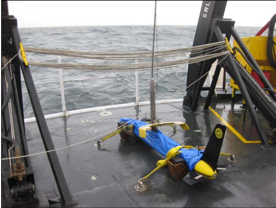
Figure 7: Towed Klein 5000 Side Scan Sonar on Fairweather
