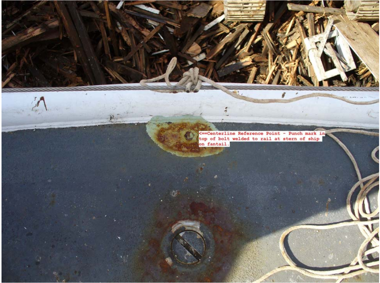
CENTERLINE STERN REFERENCE POINT
