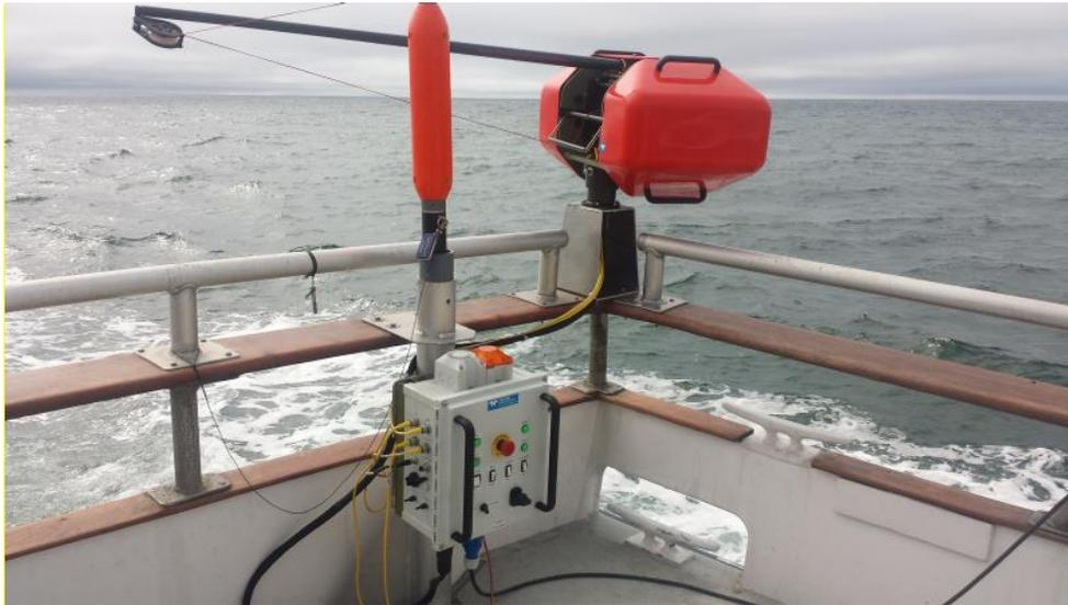
*Figure 3 – Oceanscience RapidCAST with Valeport SV sensor on the Q105.*
