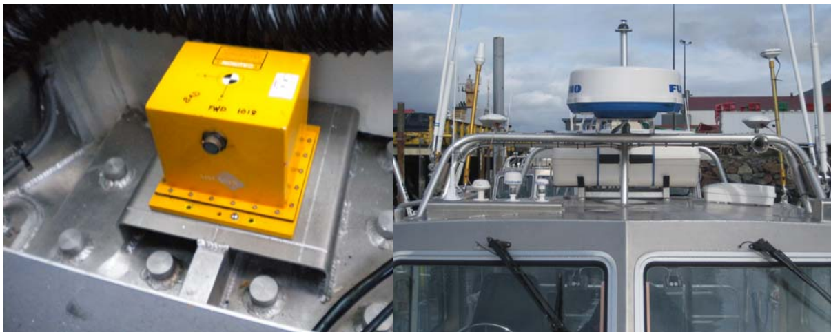
Figure 15: Vessel Reference Point (Top of POS/MV IMU) & Primary GNSS Antenna (port side).
