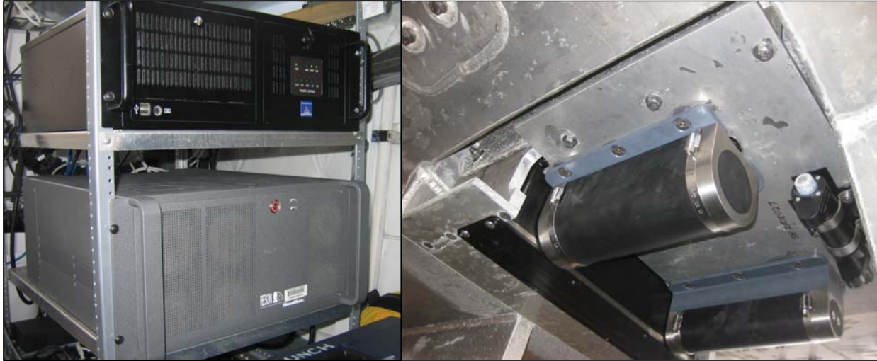
Figure 5: Reson 7125SV on a Fairweather Launch
