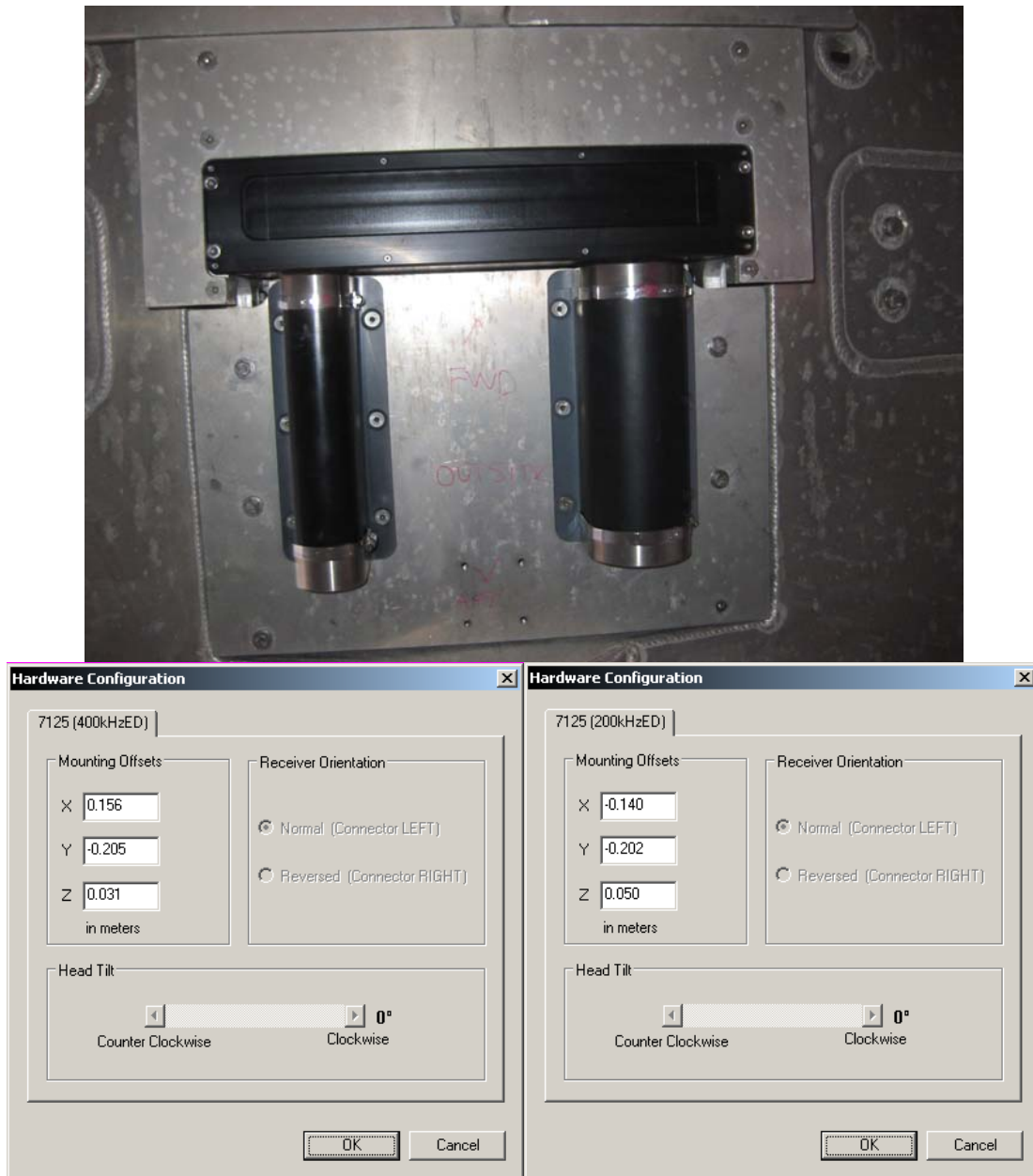
Figure 16: Reson 7125 sonar mounting with 400kHz and 200kHz offsets respectively.
