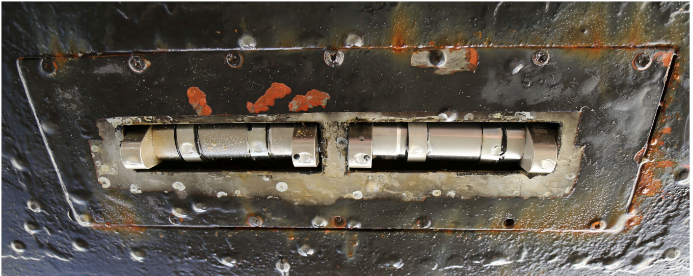
Figure 10: Dual SVP 70s mounted in Rainier's multibeam sonar transducer gondola.
