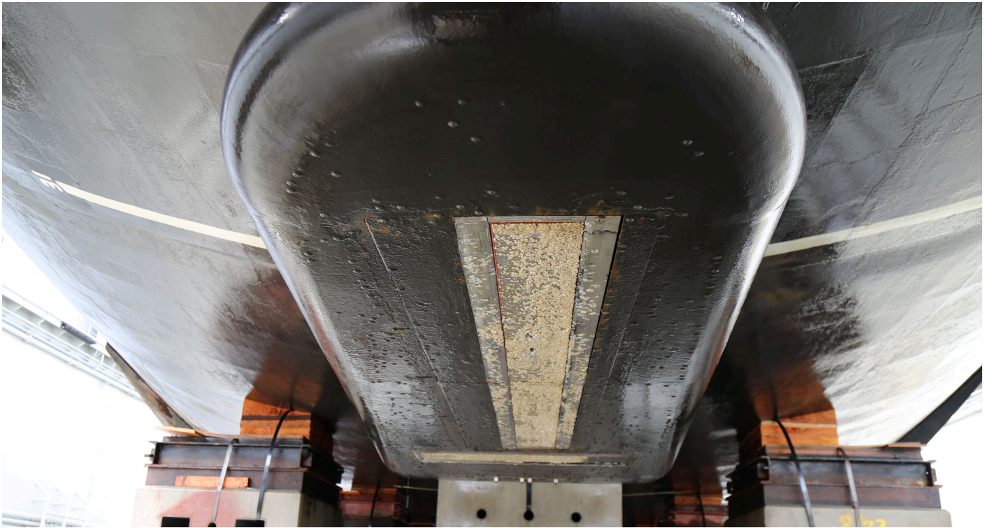
Figure 4: Kongsberg EM710 sonar transducer housing on Rainier (S221).
