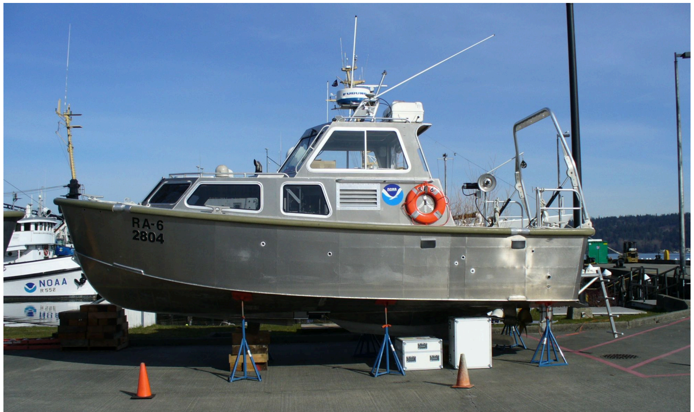
Figure 3: Rainier survey launch RA6 (2804) on blocks for her NGS offsets survey at the NOAA Western Regional Center, Sand Point, Washington.
