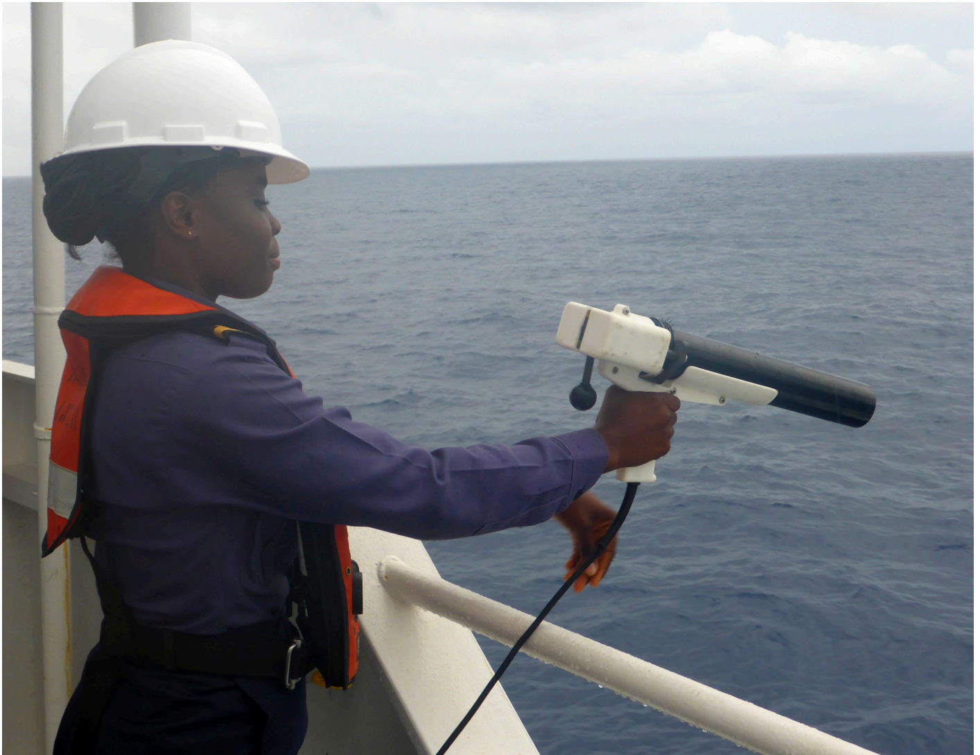
Figure 11: An XBT being deployed off the bridge wing of Rainier with a LM-A3 hand launcher.
