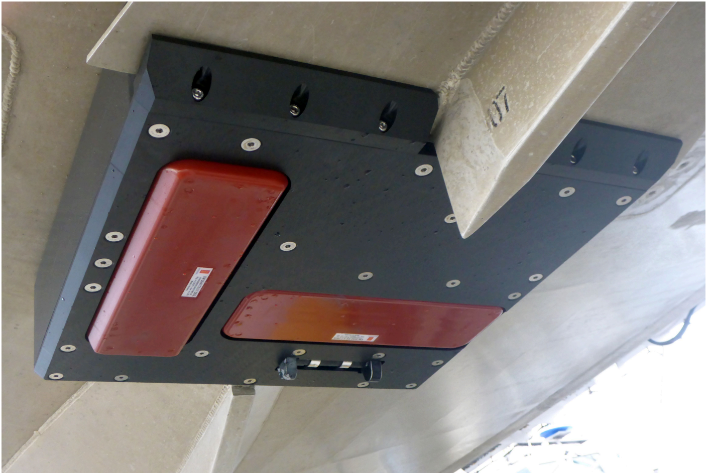
Figure 6: The Kongsberg EM2040-07 mounted on survey launch 2803.
