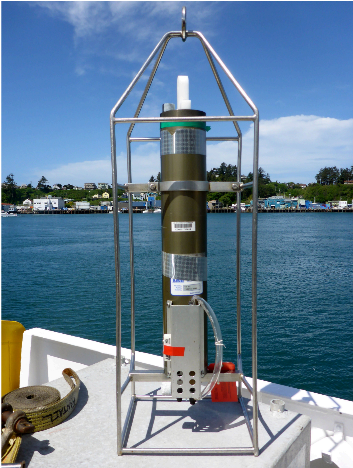
Figure 8: The SEACAT SBE 19 profiler. Note the band of electrical tape around the housing at the top of profiler marking this as the "green" CTD.
