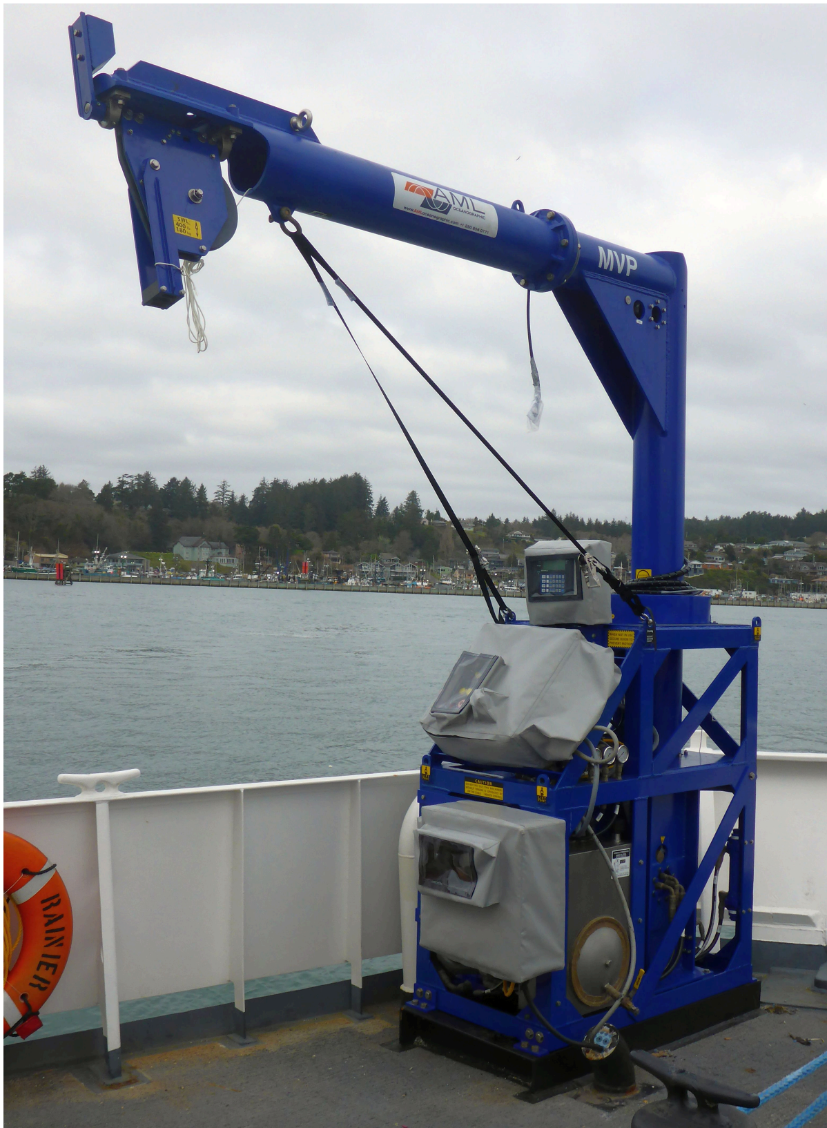
Figure 7: The MVP200 newly returned from a factory refurbishment.
