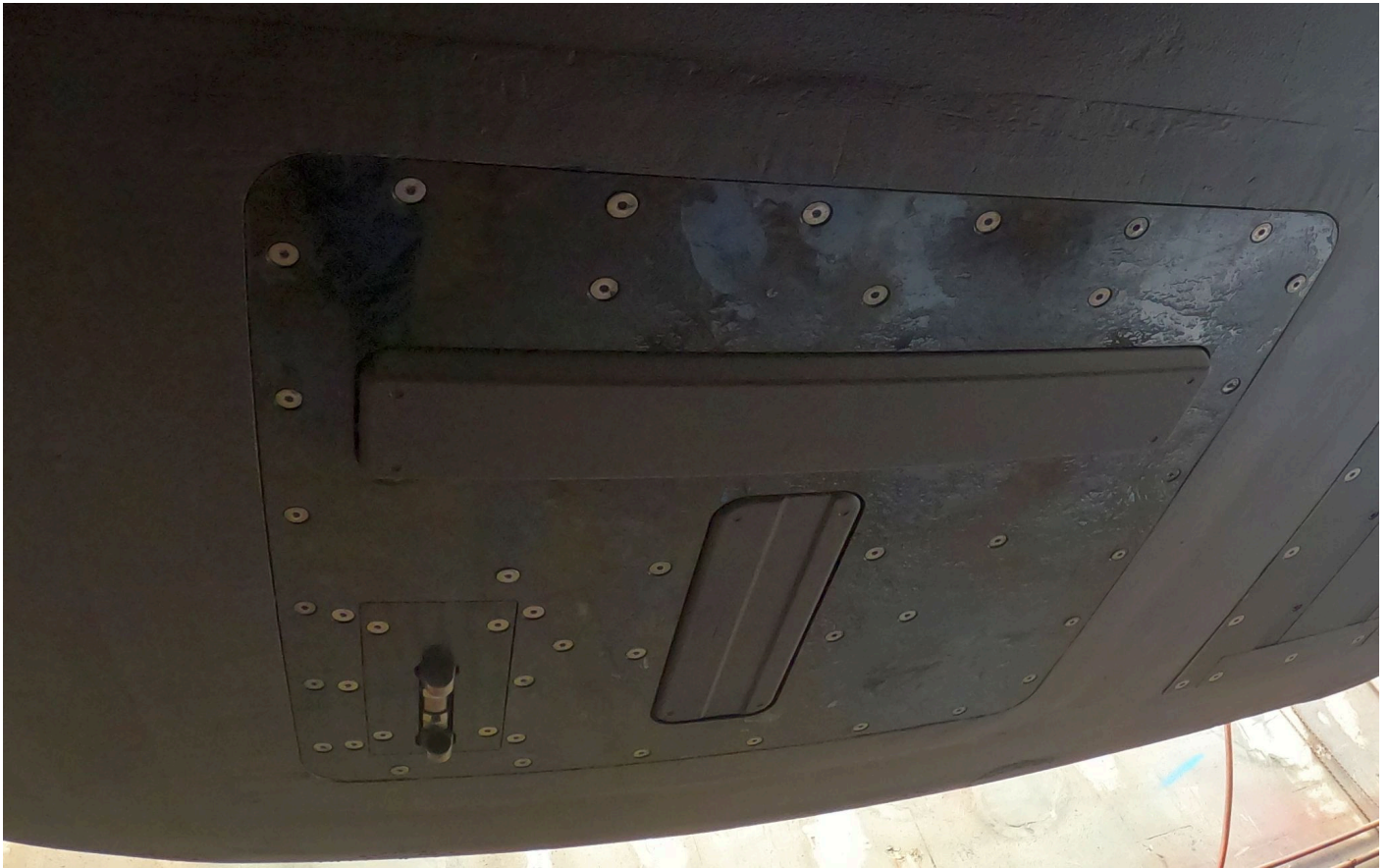
Figure 6: The Kongsberg EM2040-4 MKII TX and RX transducers as mounted in Rainier's sonar gondola.
