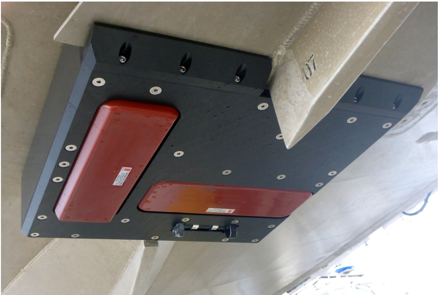
Figure 4: The Kongsberg EM2040-07 TX & RX transducers as mounted on one of Rainier's hydrographic survey launches.
