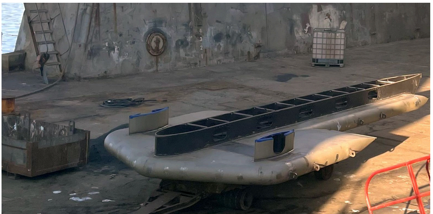
Figure 5: The "hammerhead" gondola built to house the EM304 and EM2040 transducers being prepped for installation on Rainier.
