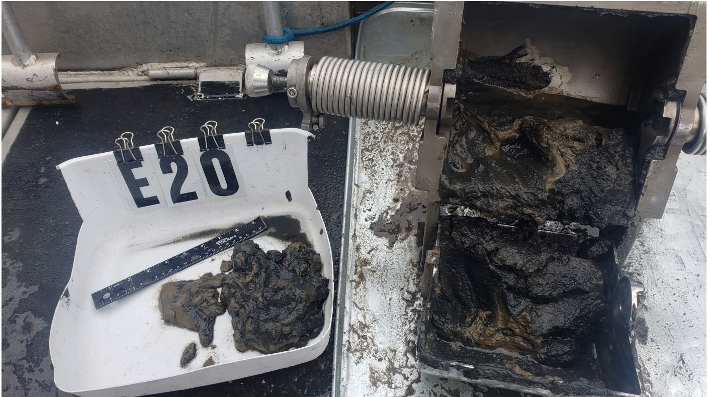
Figure 13: 860-A10 Shipek Sampler in use for bottom sample collection in H13256
