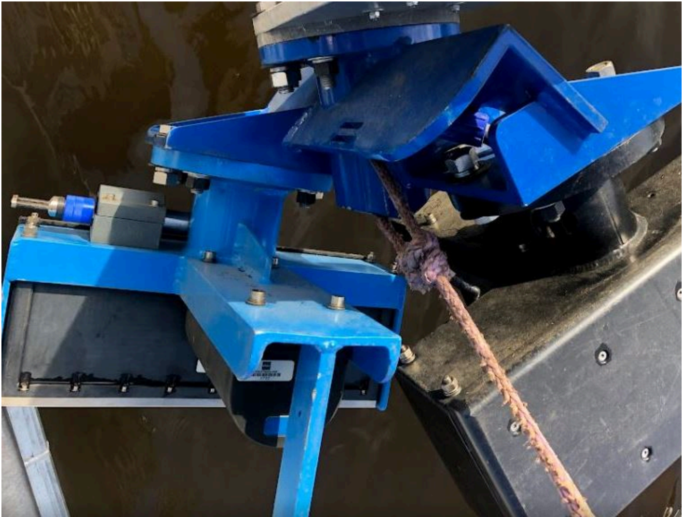
Figure 12: AML Micro•X installed on a dual head R2Sonic 2024 custom mount
