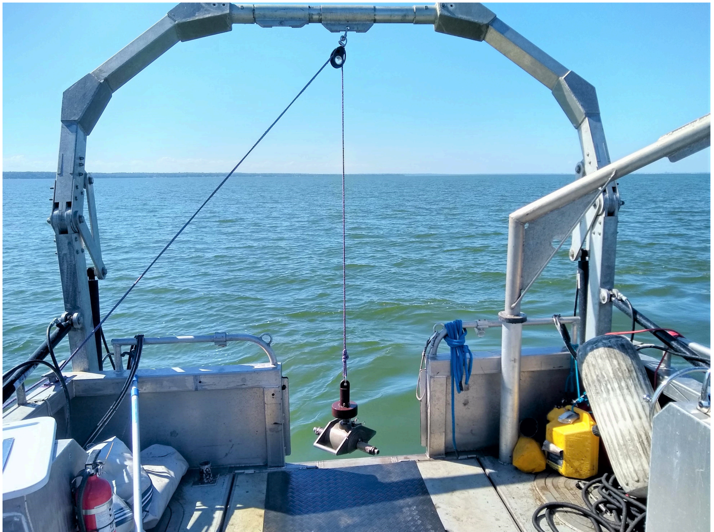
Figure 21: Shipek Grab in use for bottom sample collection
