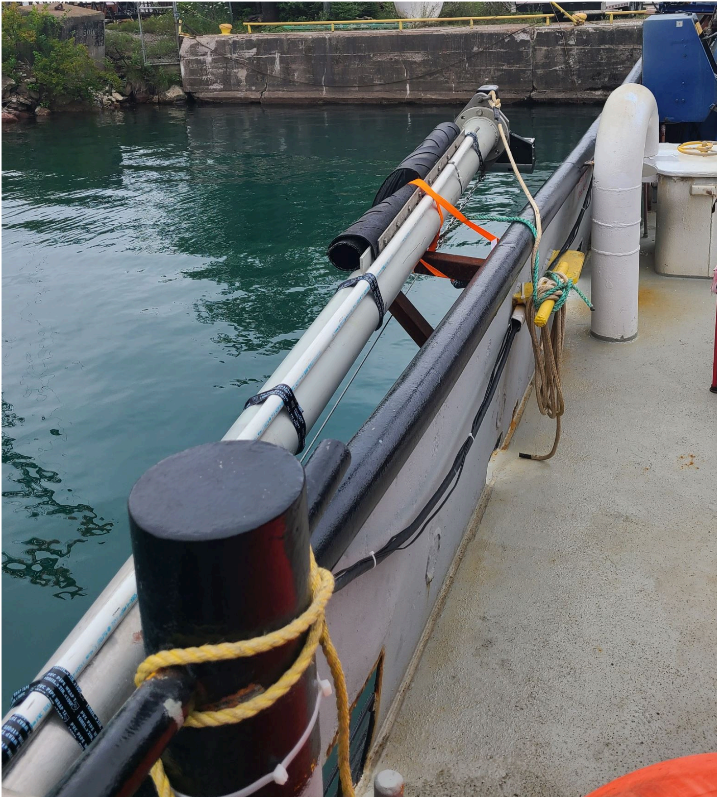
Figure 4: SeaBat T50-R transducer mounted on the MV Northstar Challenger transducer pole.
