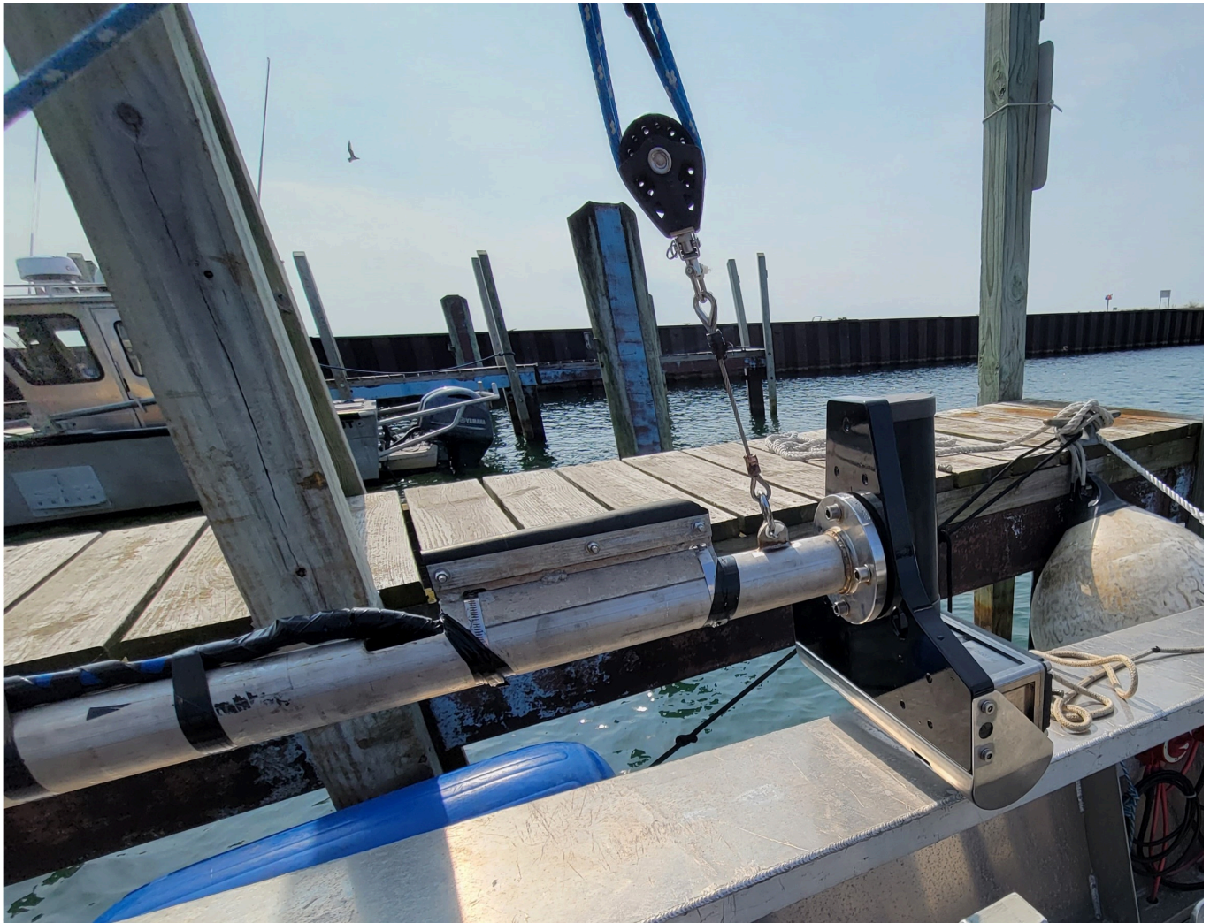
Figure 5: SeaBat T50-R transducer mounted on the RV North Cove transducer pole.
