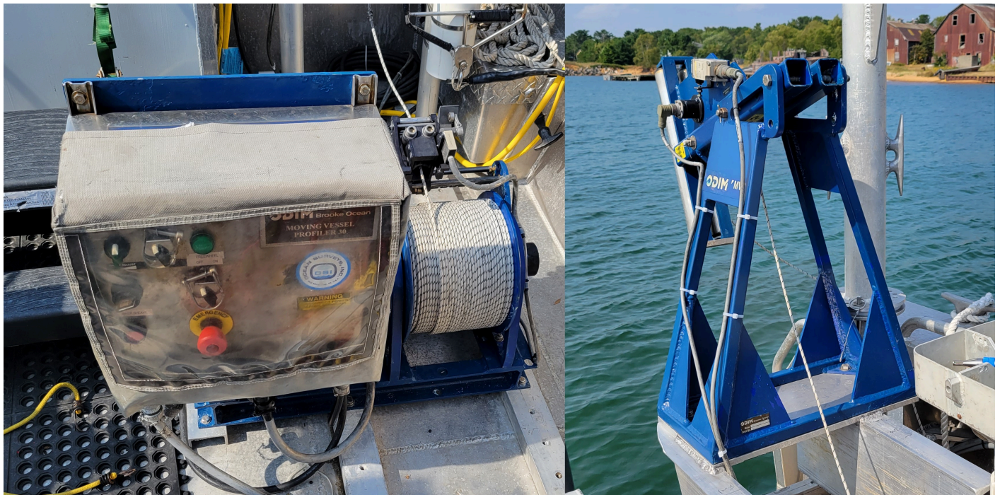
Figure 14: MVP30 Moving Vessel Profiler mounted on the port quarter of the RV North Cove.
