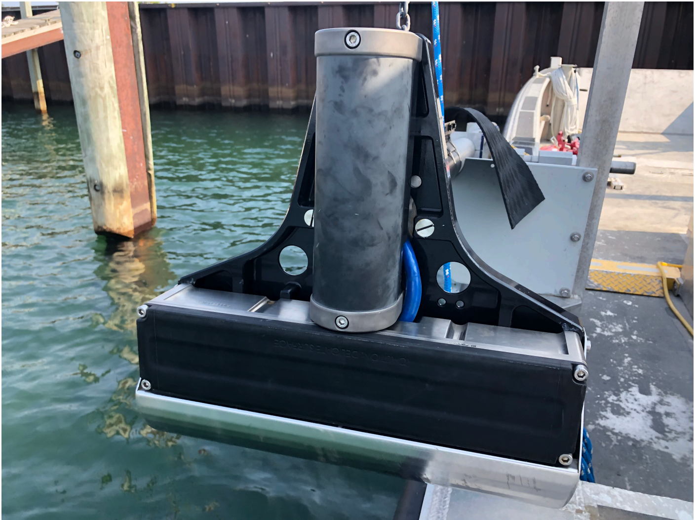
Figure 6: SeaBat T50-R transducer mounted on the RV H.F. Stout transducer pole.
