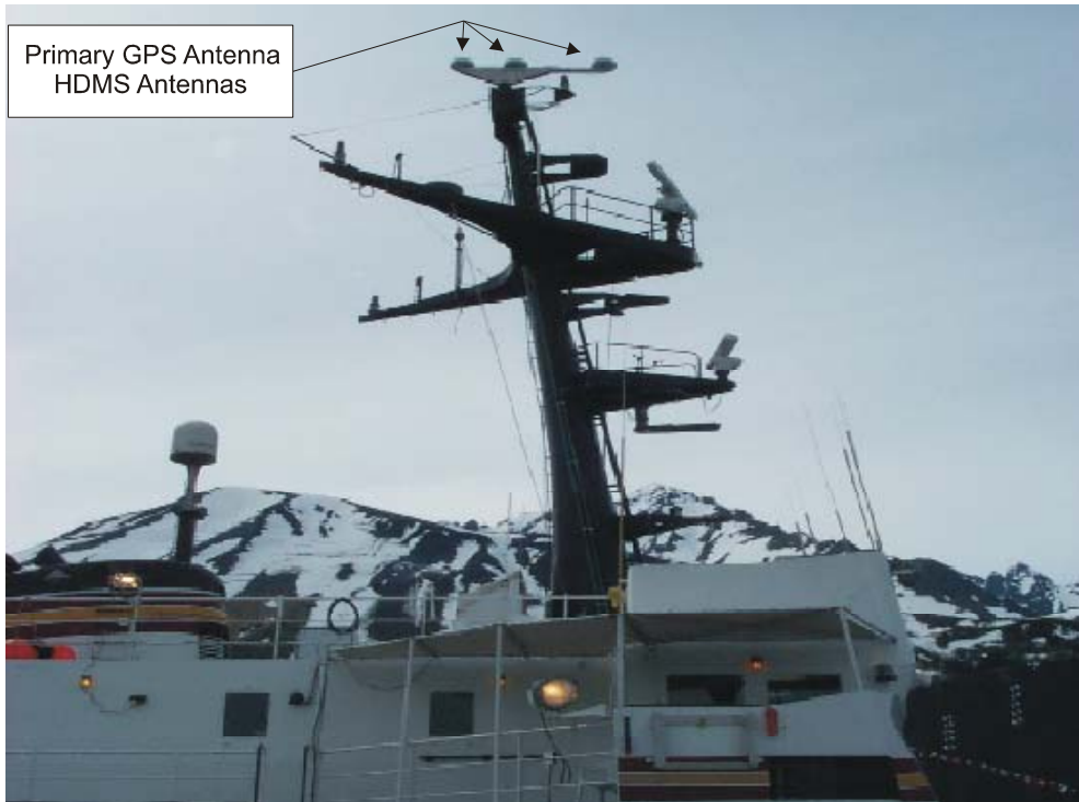
Figure B-3 Primary GPS and HDMS Antennas
