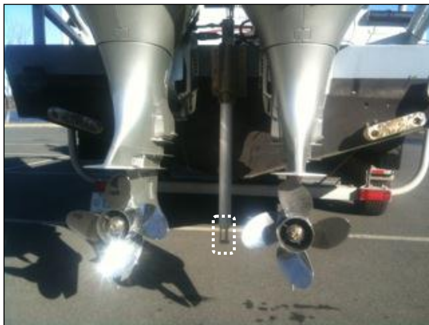
Figure 5: Surface Sound Speed Digibar Installation
