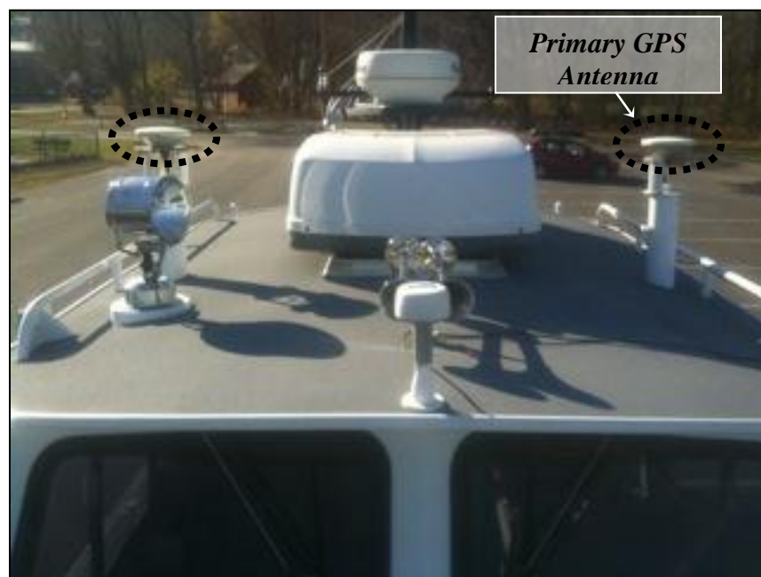
Figure 2: POS/MV Antenna Installation
