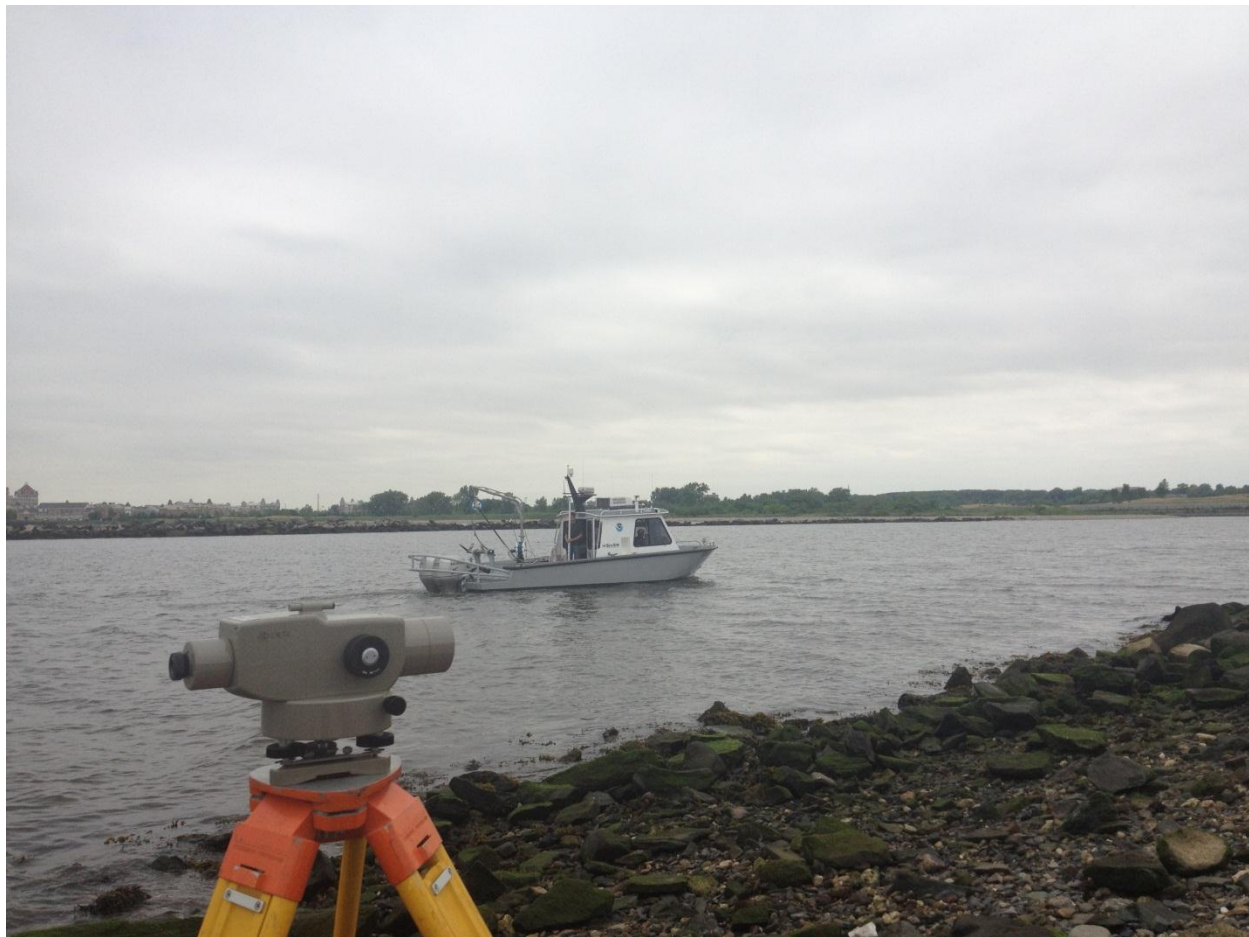
Figure 14: Dynamic Draft Optical Level Setup
