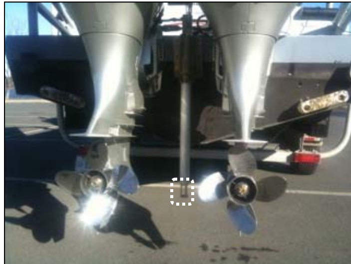
Figure 4: Surface Sound Speed Digibar Installation
