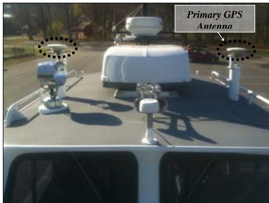
Figure 2: POS/MV Antenna Installation
