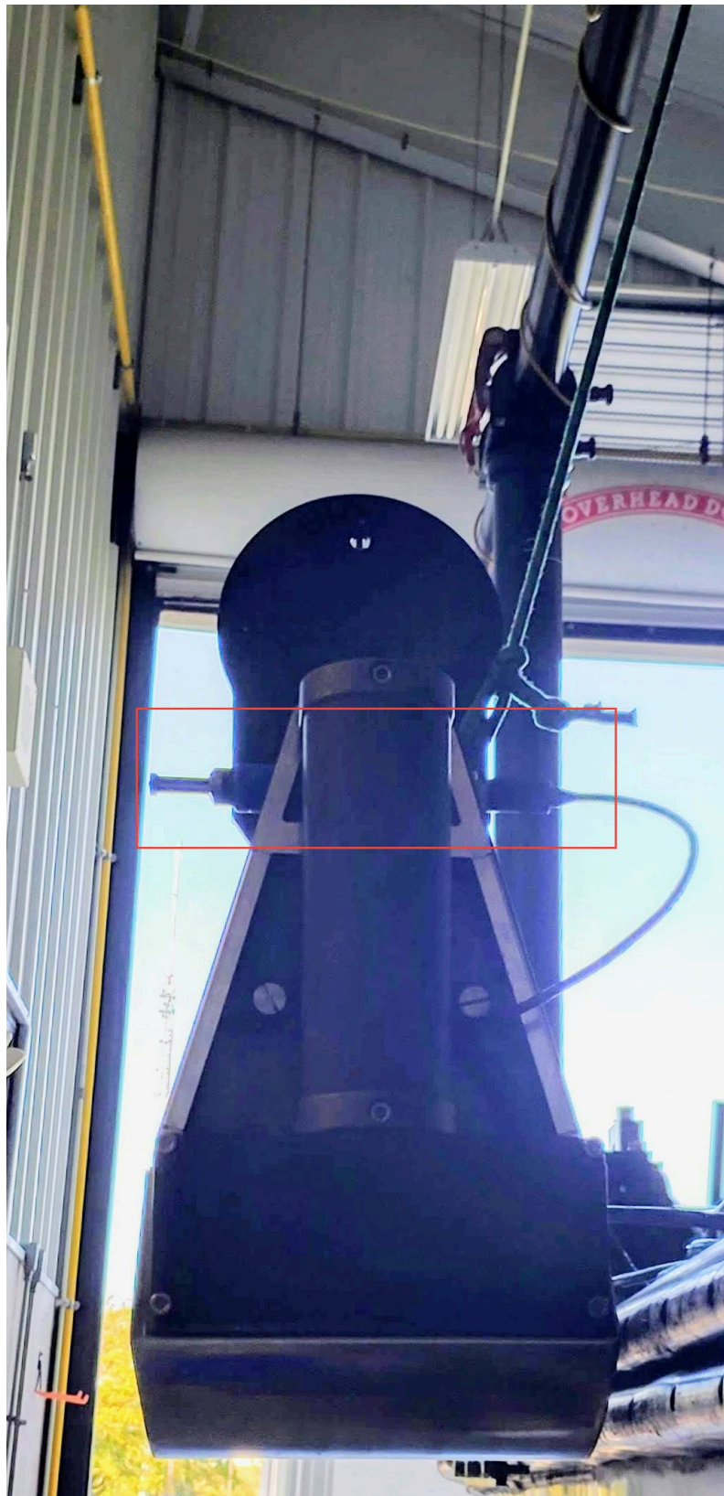
Figure 6: Underside view of MBES mount. Note the SV sensor highlighted in red.
