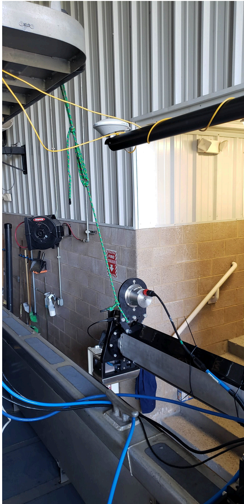
Figure 9: Topside view of MBES and IMU. Note the very small lever arm between the two sensors.
