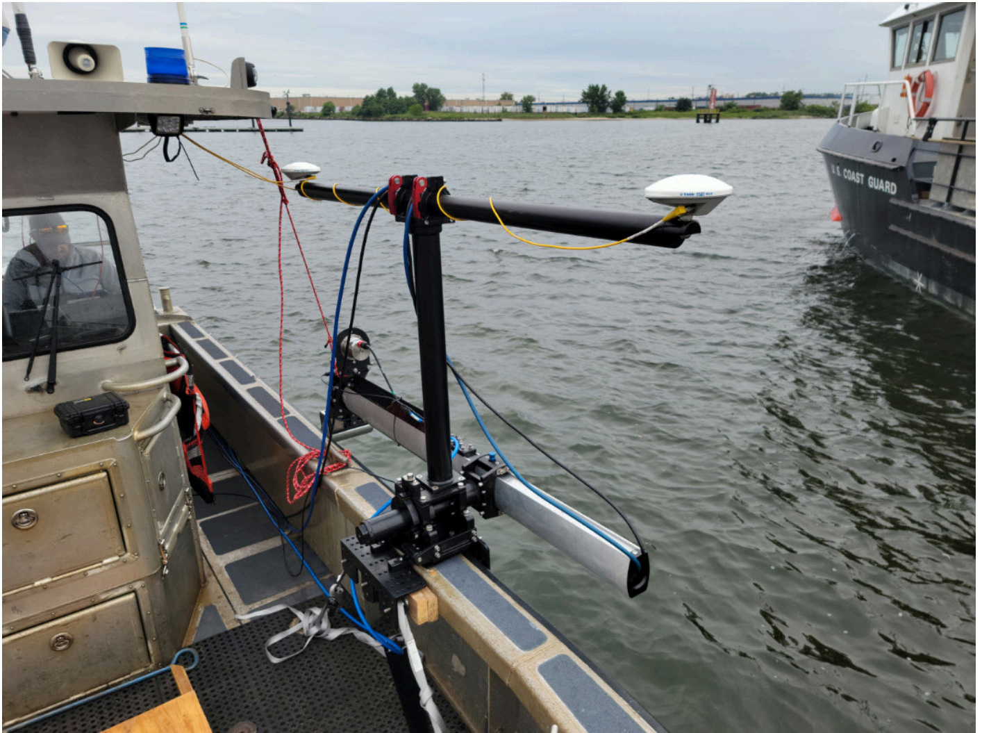
Figure 7: Close up of the USM pole kit with GPS mast and sonar Z-pole.
