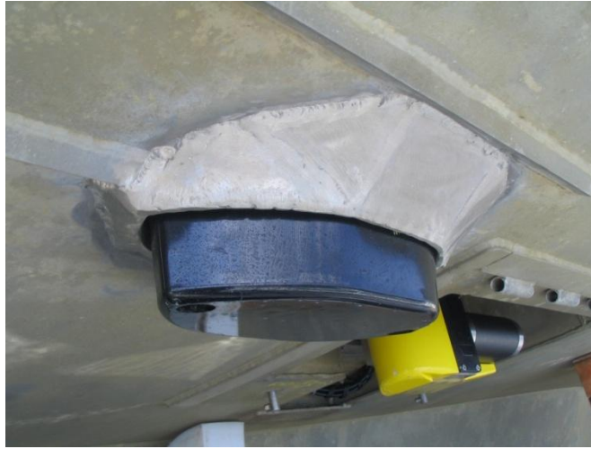
Figure A-3 - Odom Vertical Beam on 3101 / 3102.
