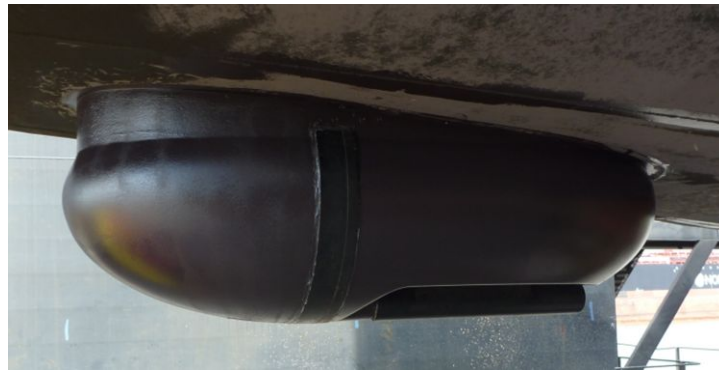
Figure 6: 7111 mount and fairing. Sonar is located forward on the starboard hull.
