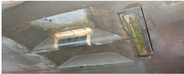
Figure 3: 7125 Housing flush mounted on hull
