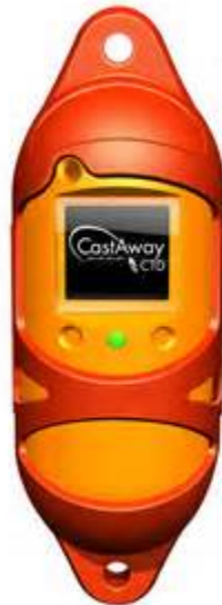
Figure 5: SonTek CastAway CTD.
