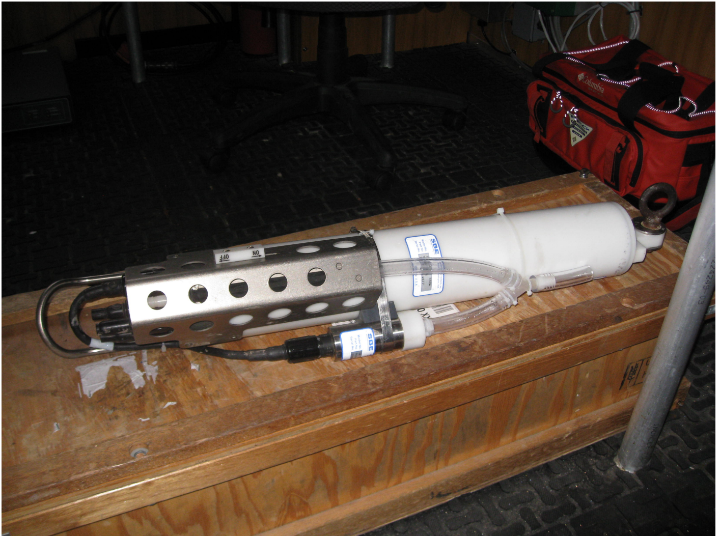
Figure 11: R/V BAY HYDRO II's SeaBird 19plus CTD.
