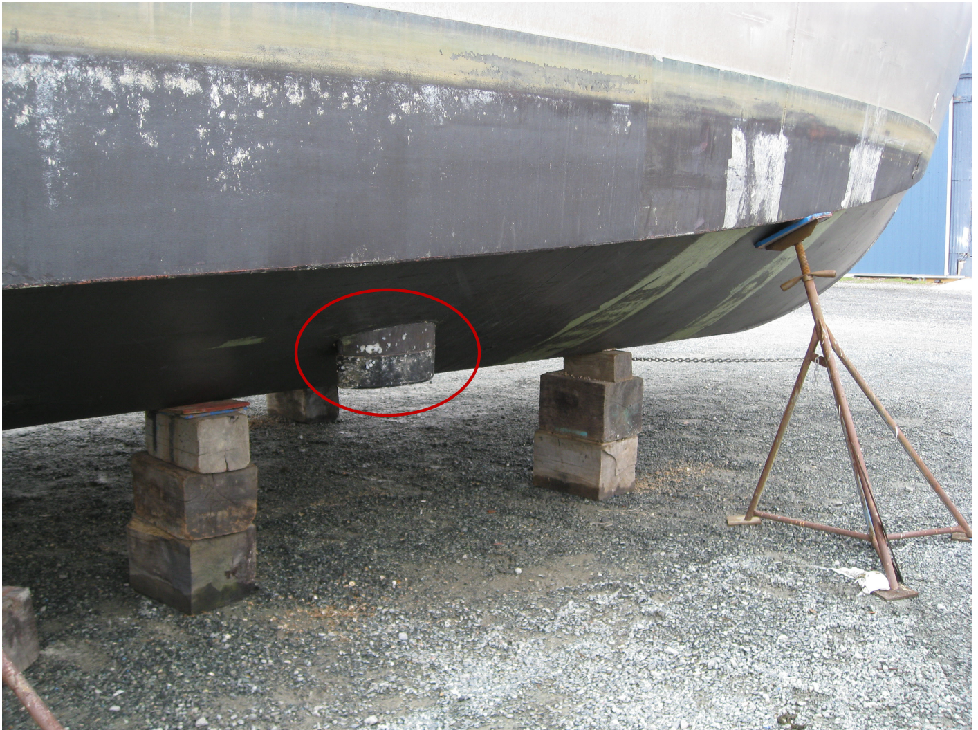
Figure 5: R/V Bay Hydro II's hull mounted starboard SBES sonar.
