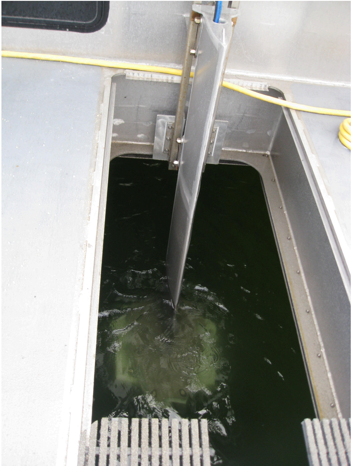
Figure 4: Kongsberg EM2040C-DH housing and sonar in the deployed position.
