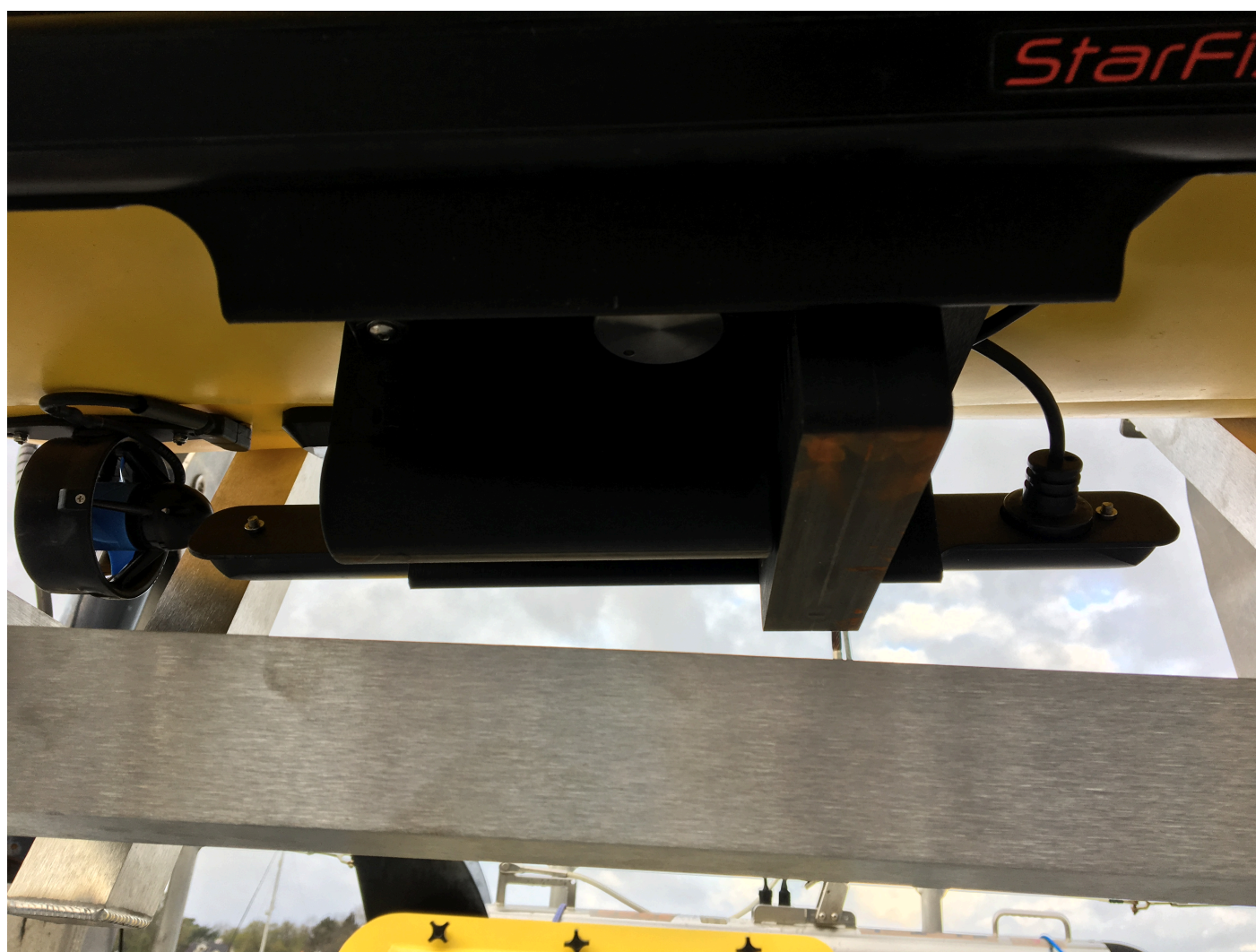
Figure 3: PicoMBES installed on ASV007.
