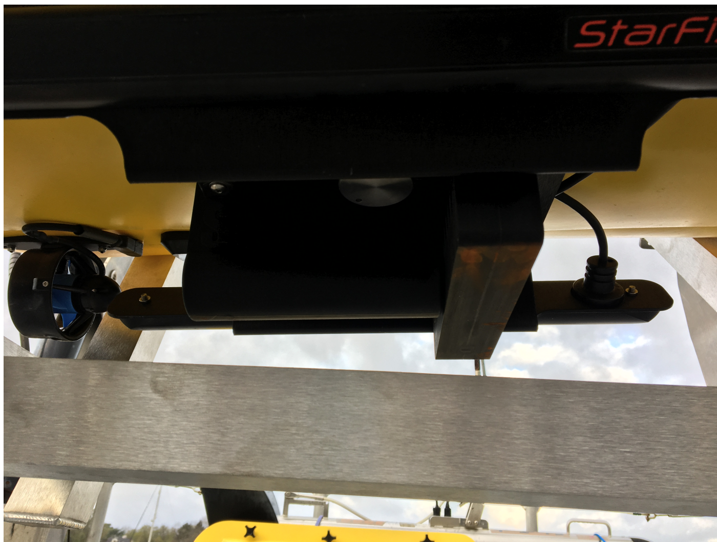
Figure 3: PicoMBES installed on ASV007.
