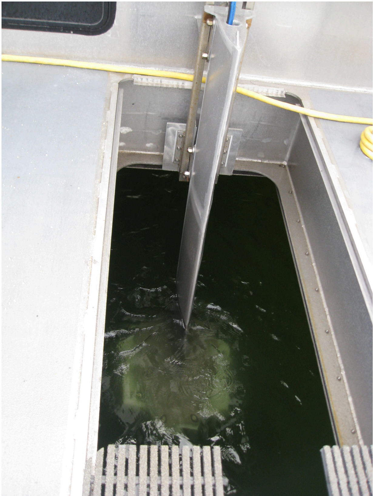
Figure 3: Kongsberg EM2040C-DH housing and sonar in the deployed position.
