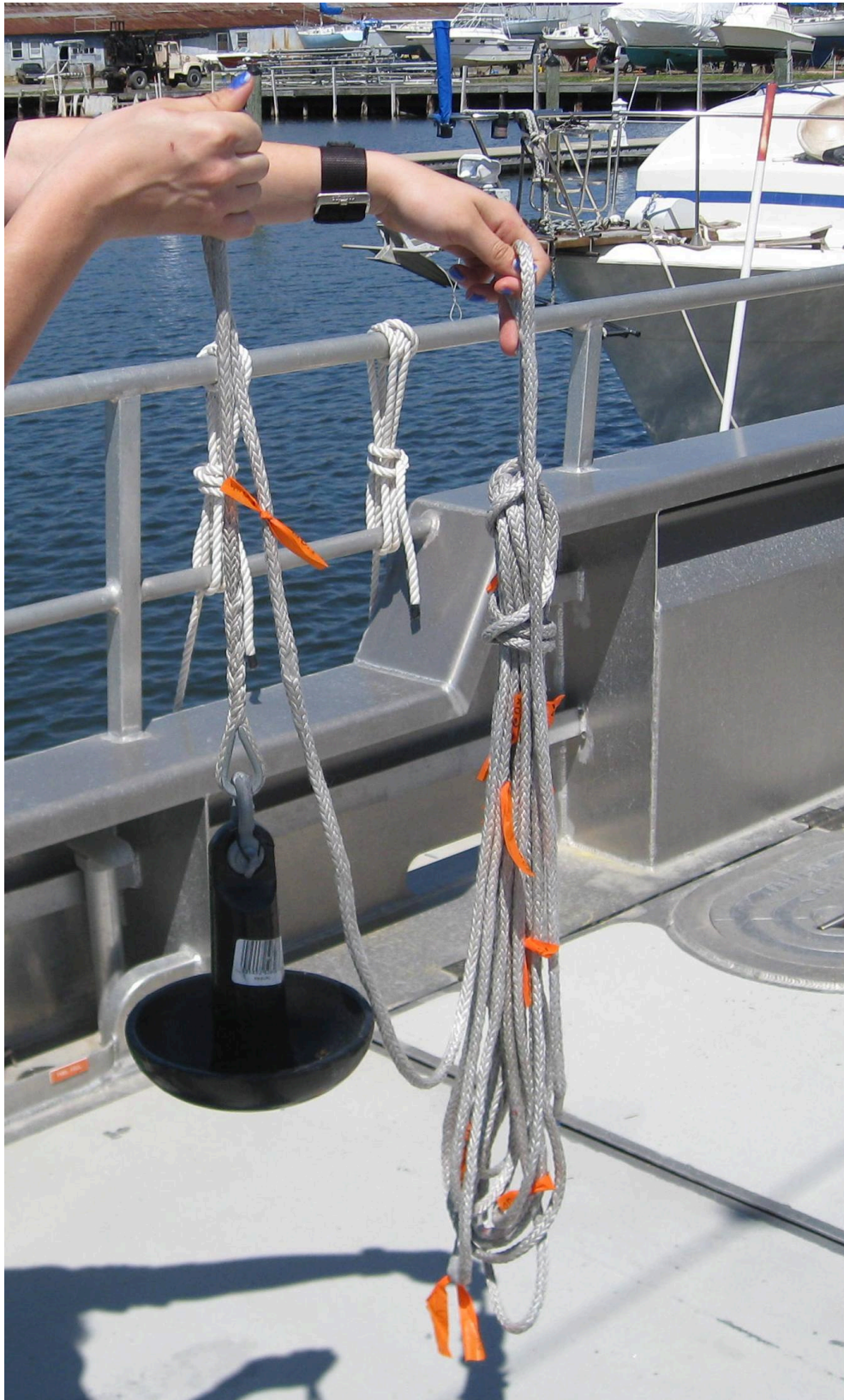
Figure 8: Bay Hydro II's non-traditional lead-line with orange meter incrementation.
