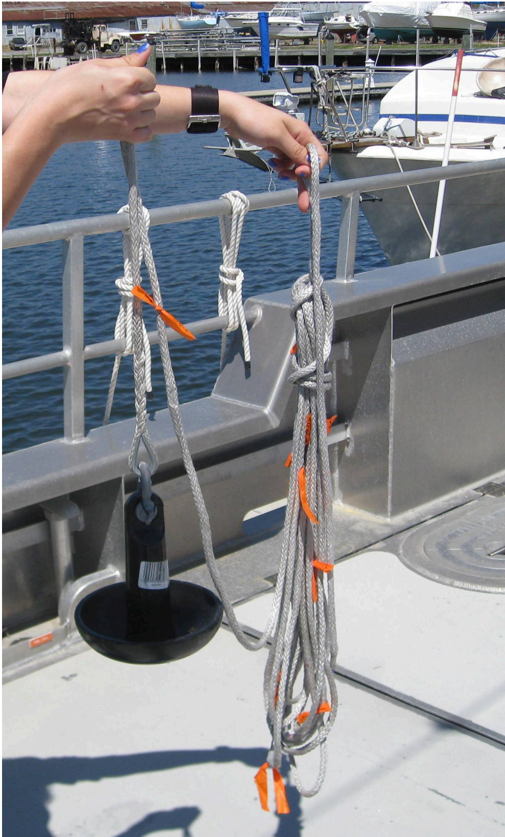
Figure 5: Bay Hydro II's non-traditional lead-line with orange meter incrementation.
