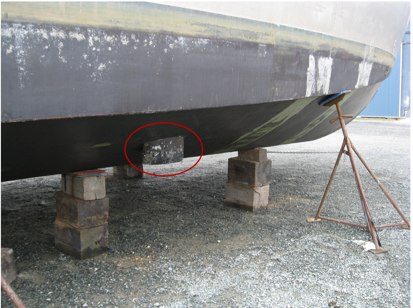
Figure 4: R/V Bay Hydro II's SBES sonar mounted outboard on the starboard hull.
